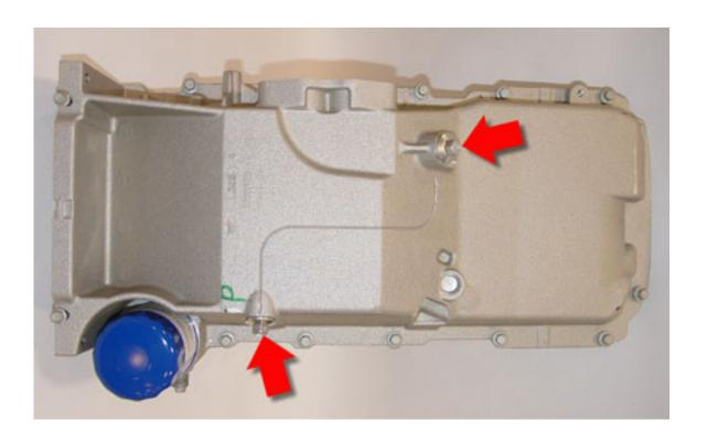
Once the oil has been drained from the engine and reservoir, replace the engine oil filter with a new PF48 oil filter and tighten to 25 Nm (18 lb ft).
