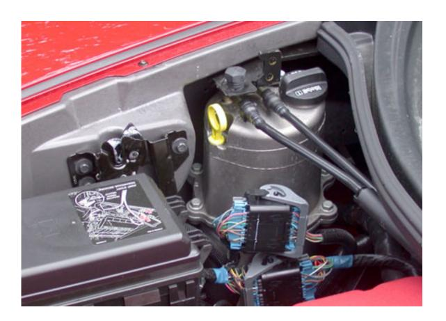
Additionally, oil aeration is lower in a dry sump system, because the oil spends less time in the presence of the crankcase windage. Oil delivered to the bearings is typically superior to that of a wet sump system.
