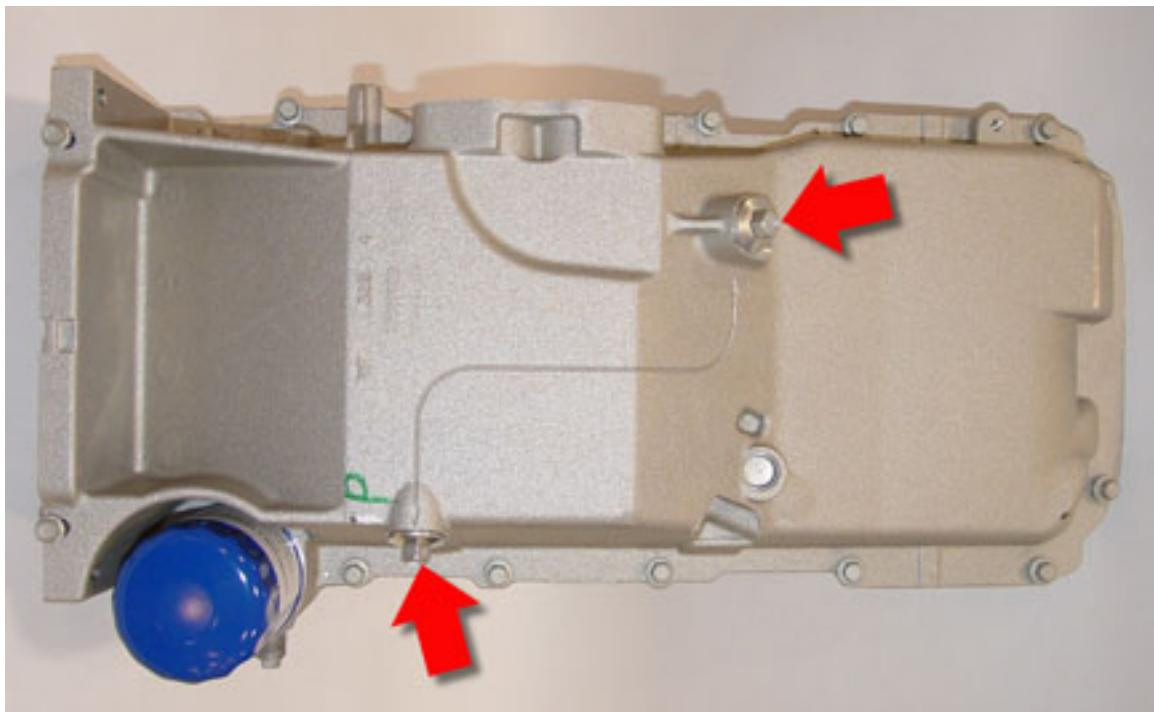
Once the oil has been drained from the engine and reservoir, replace the engine oil filter with a new PF48 oil filter and tighten to 25 Nm (18 lb ft).
