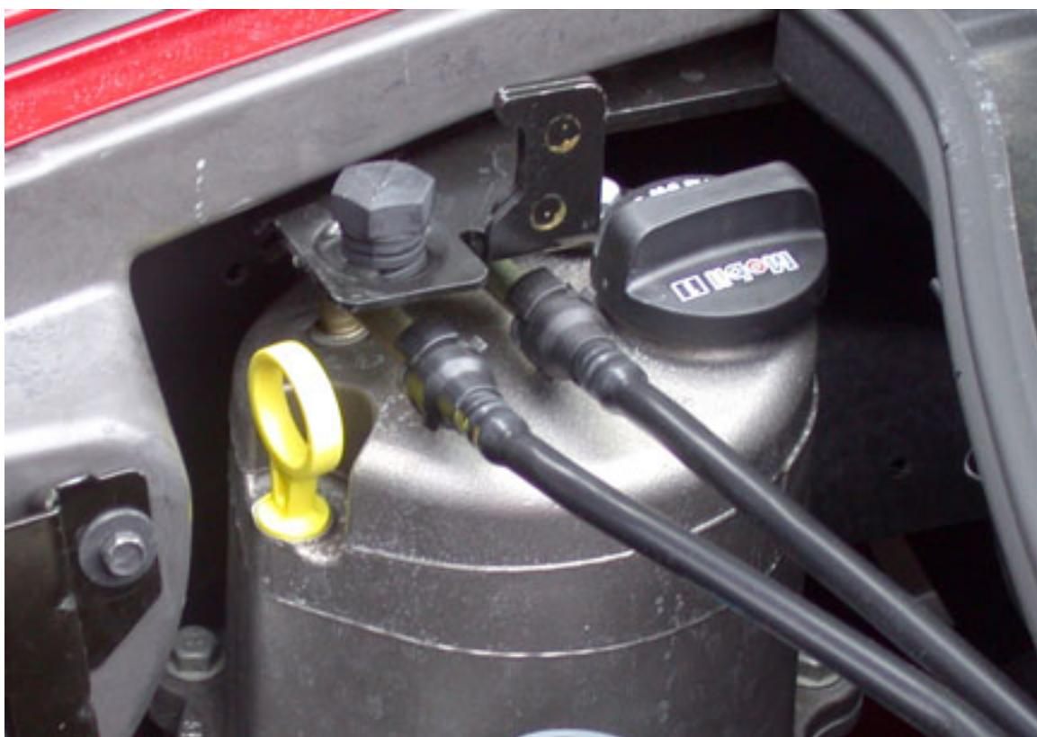
**TIP:** Do not overfill the reservoir, as this may result in excessive oil consumption. Oil levels above the crosshatched area may degrade lubrication.
