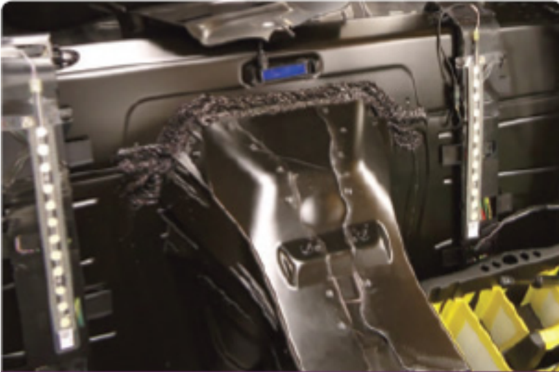
Bulkhead Limit Switch located on the left and right body harness conduit.
