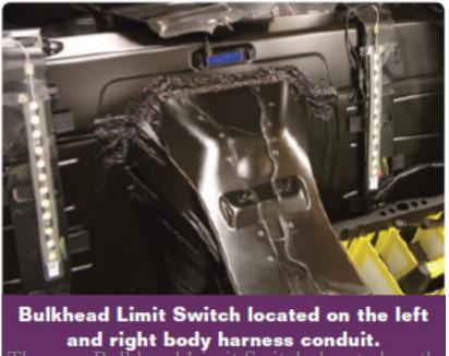
The new Bulkhead Limit Switch, located on the left and right body harness conduit, is used in both seating positions and acts to prevent damage to the body harness and seatback covers when the seat or seatback is moved in a rearward direction. When this switch is active (any time pressure is detected against the rear bulkhead/carpet area directly behind the seats), power seat movement is limited to movements that will bring the seat/seat-back forward.
