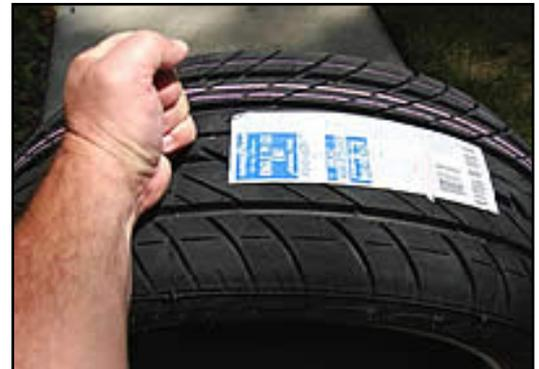
**Additionally, most of the casing, including the tread itself will be more stiff than that of regular tires. This stiffness is easily felt when handling any run-flat.**
