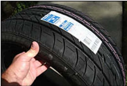
**One physical characteristic of any run-flat is a sidewall that is more stiff than that of a non-run flat tire.**
