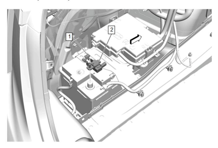
If a battery is improperly charged, the Battery Sensor Learn will be required to calibrate the Battery Sensor Module. With the ignition off, let the vehicle rest for a minimum of four hours without any interruptions (opening a door, using the key fob, etc.). Verify if the battery SOC is 70 percent or greater using GDS 2 before attempting to continue with an OTA update.
