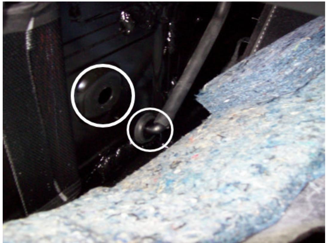
3. The drain tube may be partially or fully disconnected from the body sheet metal as shown.
