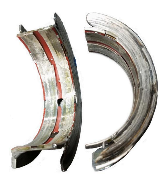
1. Inspect the thrust bearing for wear on one side and crankshaft on the corresponding mating surface. The graphic above shows an example of a damaged thrust bearing.
