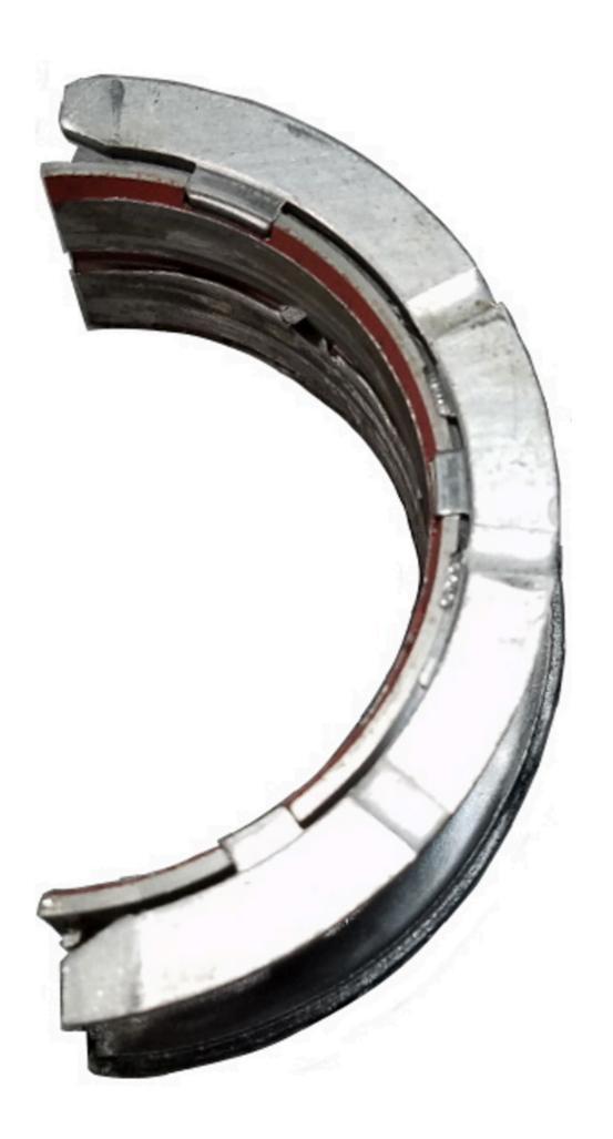
Example of a good thrust bearing face.
