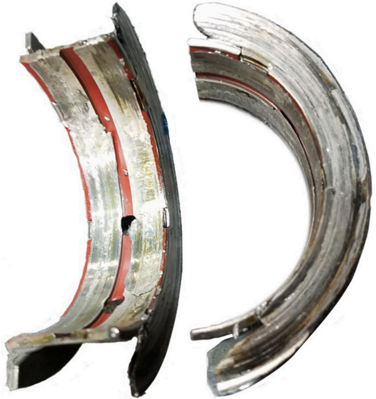
1. Inspect the thrust bearing for wear on one side and crankshaft on the corresponding mating surface. The
