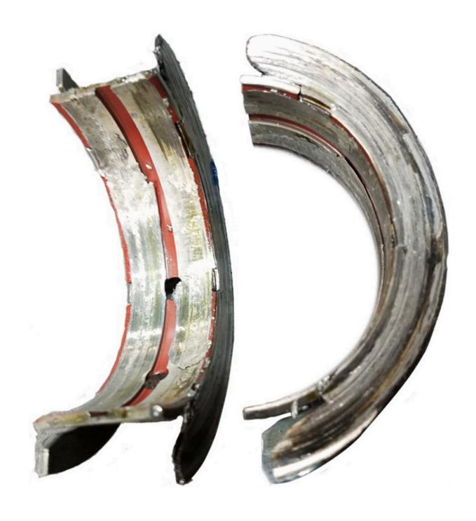
1. Inspect the thrust bearing for wear on one side and crankshaft on the corresponding mating surface. The
