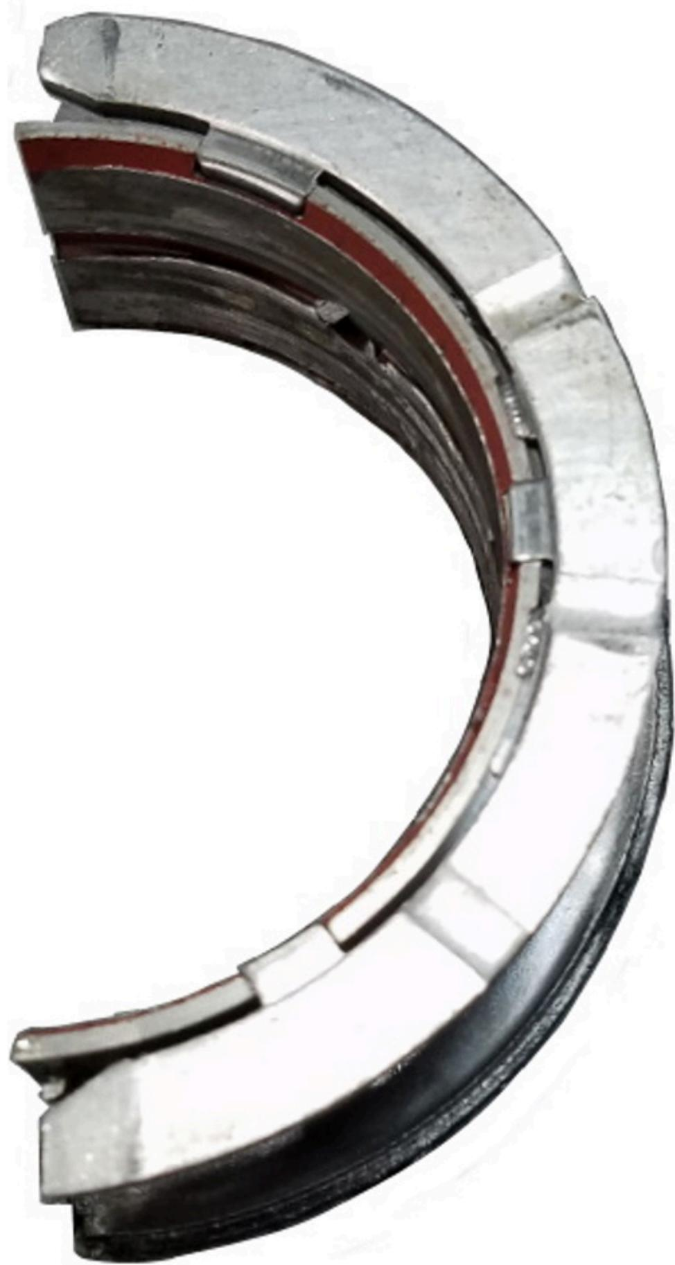
*Example of a good thrust bearing face.*
