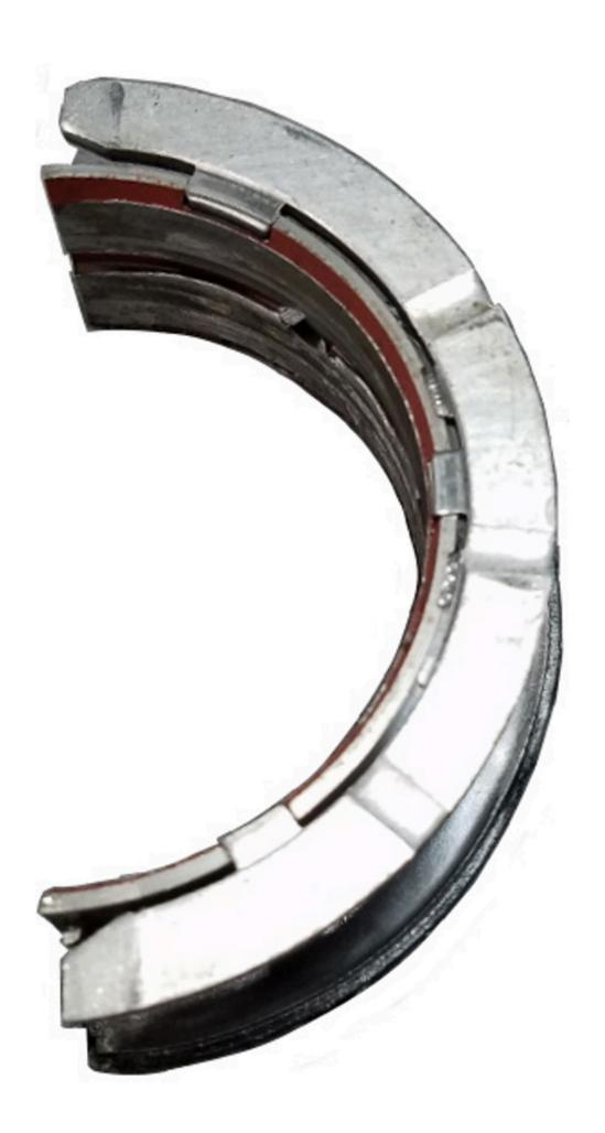
Example of a good thrust bearing face.
