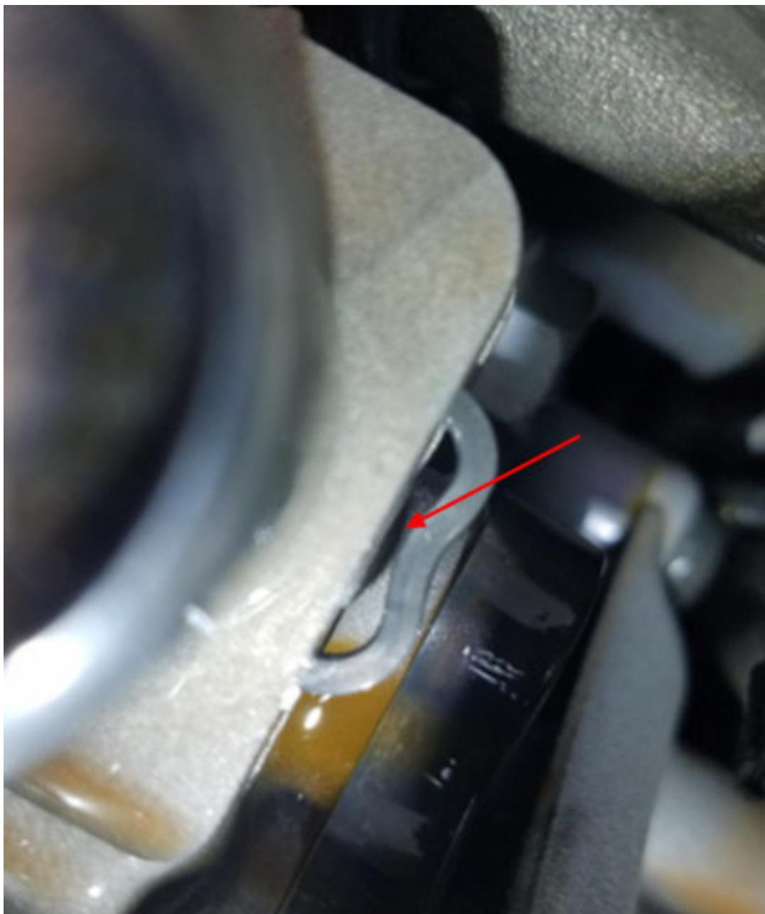
1. When the retainer is installed, there should be about 2 to 3 mm of clearance between the retainer and the oil pump body as shown above.
