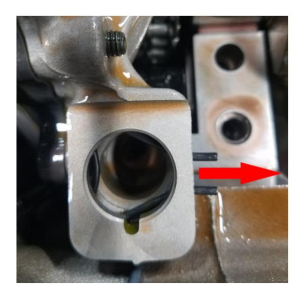
**Note:** Remove the existing oil pressure control valve retainer by pulling towards the rear and discard. You will be installing a newly designed retainer during installation.
