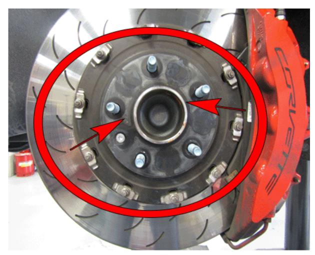
Using 3M red Scotch-Brite 7447 pad or equivalent with approved brake cleaner (ex. Part number 19370705 (U.S.), 88901247 (Canada)), wipe the wheel mounting surface of the rotor (brake rotor top hat) and the wheel pilot at the center of the rotor, removing any residual grey or black material that has accumulated on the rotors.
