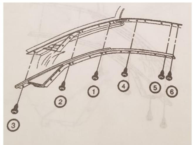
**16.** Loosely install the side reveal molding screws. Wrap 3M calk around each screw to create a waterproof seal.
