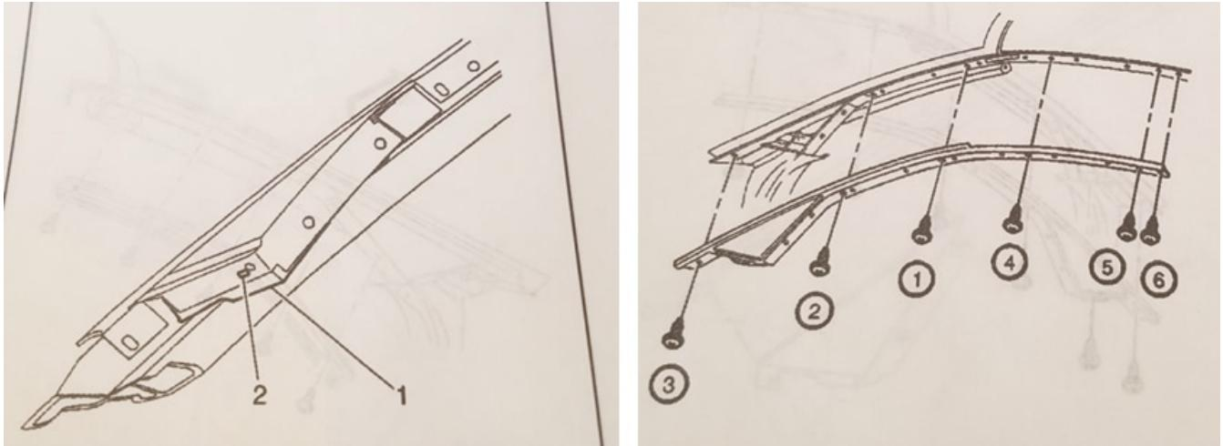
16. Loosely install the side reveal molding screws. Wrap 3M calk around each screw to create a waterproof seal.
