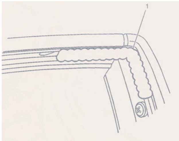
27. Apply three parallel 2 inch long beads of sealant (1) to the forward end of the door opening weather strip retainer and to the rear edge of the reveal molding.
