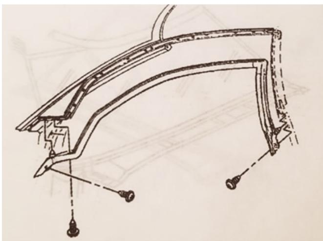
30. Install the push-in retainer (1) securing the weatherstrip to the hinge pillar reveal molding.
