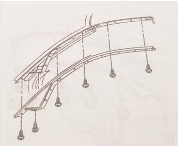
8. Remove the side reveal molding.
