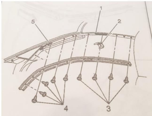
23. Tighten the side retainer to applique and windshield screws to 22 lb inch.
