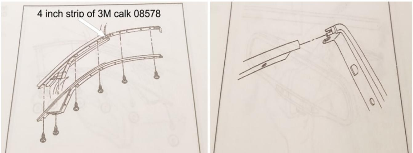
14. Install the reward end of the side reveal molding over the lock pillar upper molding.
