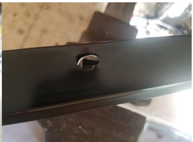
4. Carefully clean with 3M adhesive remover 08984 and remove dimples from metal retainer. Use a 3/8 drive extension mounted in a vise to set part on. Then carefully hammer to flatten part.
