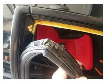
**3.** Remove the nine #2 Phillips screws that hold the weatherstrip retainer.
