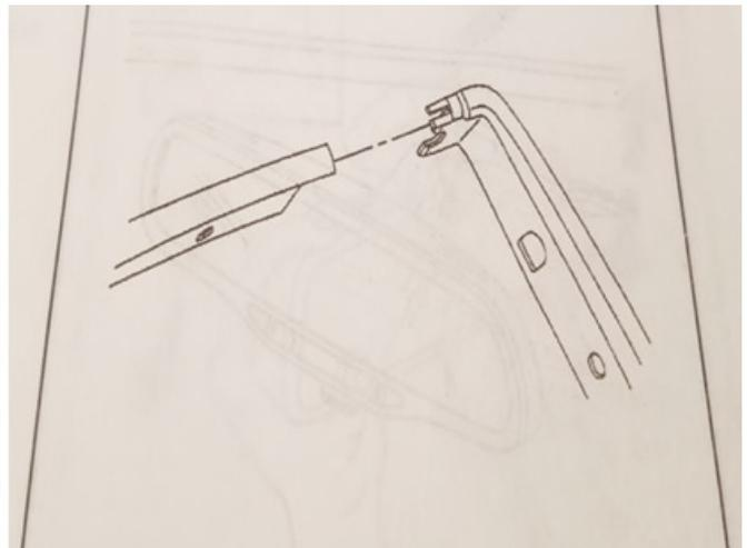
**14.** Install the reward end of the side reveal molding over the lock pillar upper molding.
