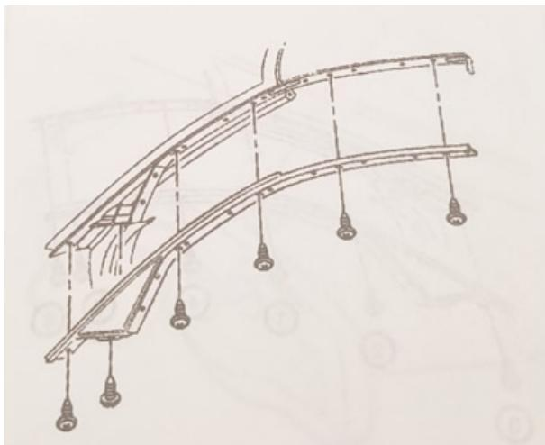
8. Remove the side reveal molding.
