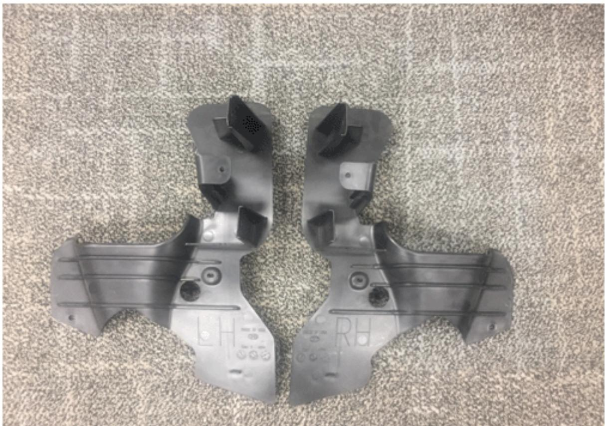
Only install the front lower control arm plastic brake cooling deflector during the PDI process.
