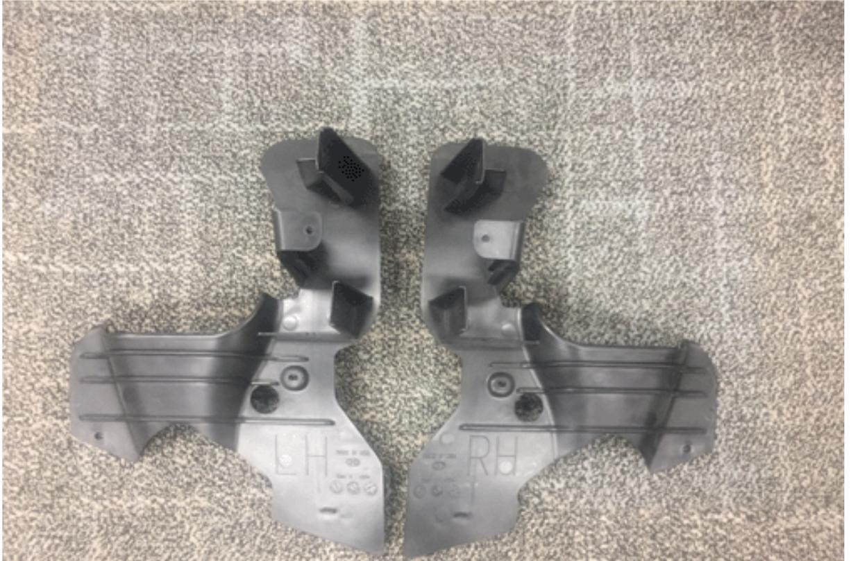
Only install the front lower control arm plastic brake cooling deflector during the PDI process.
