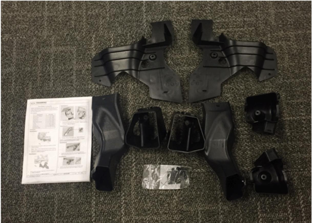
The additional brake cooling parts should be provided to the customer. The customer may want the parts installed prior to his or her track event.
