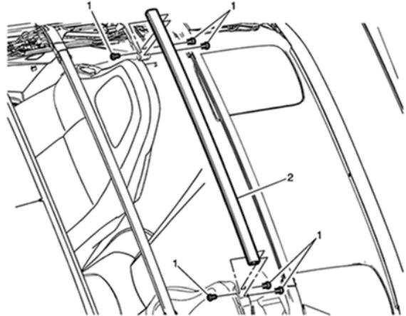
The cause of the condition may be that the fasteners (1) at the ends of the #3 Bow (2) may have lost torque.
