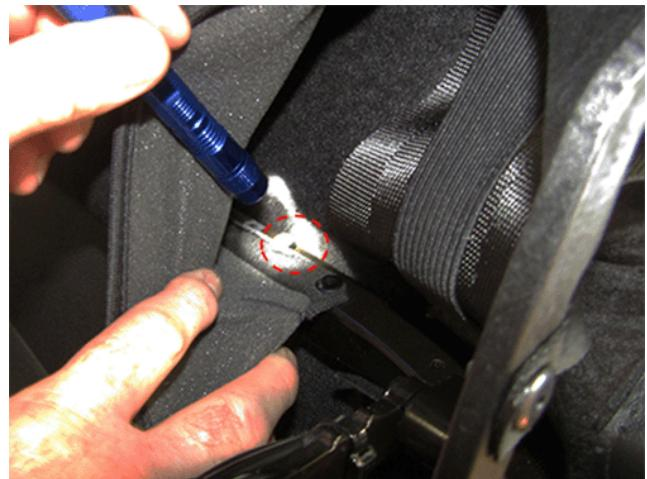
Following the Service Procedure below, remove the original smaller screws and install the new larger M6 screws referenced in the Part Table.
