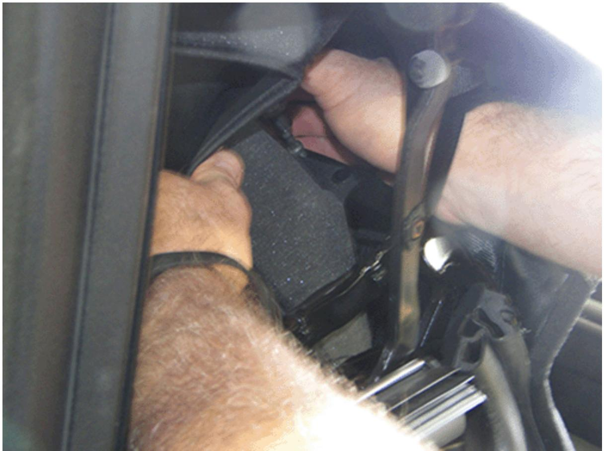
1. Position the top to best reach under the headliner to access the 3 retaining screws on each end of the #3 Bow.
