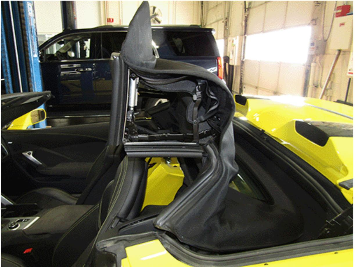
**Warning: Due to bleed off of the hydraulic pressure, the folding top will have to be supported or held in mid-position by an assistant. Manual operation of the top cannot be attempted for at least 5 minutes from the last time of activation.**
