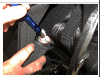
Following the Service Procedure below, remove the original smaller screws and install the new larger M6 screws referenced in the Part Table.
