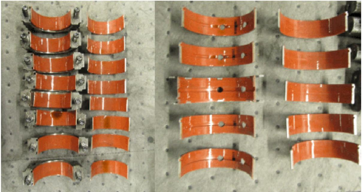
Inspect thrust bearing for wear on one side and crankshaft on that “mating” surface.
