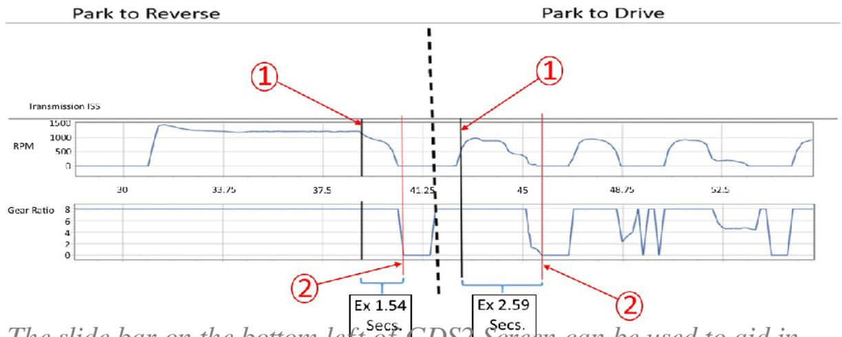
*The slide bar on the bottom left of GDS2 Screen can be used to aid in discerning time (Pt. 2 – Pt. 1) = Delayed Engagement Time.*
