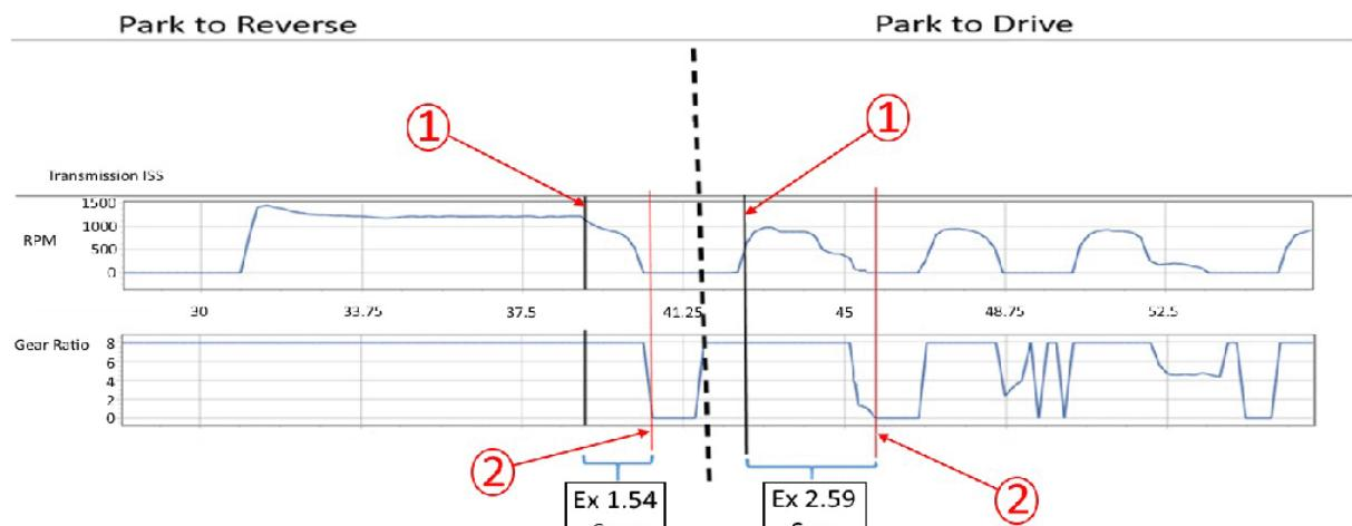
*The slide bar on the bottom left of GDS2 Screen can be used to aid in discerning time (Pt. 2 – Pt. 1) = Delayed Engagement Time.*
