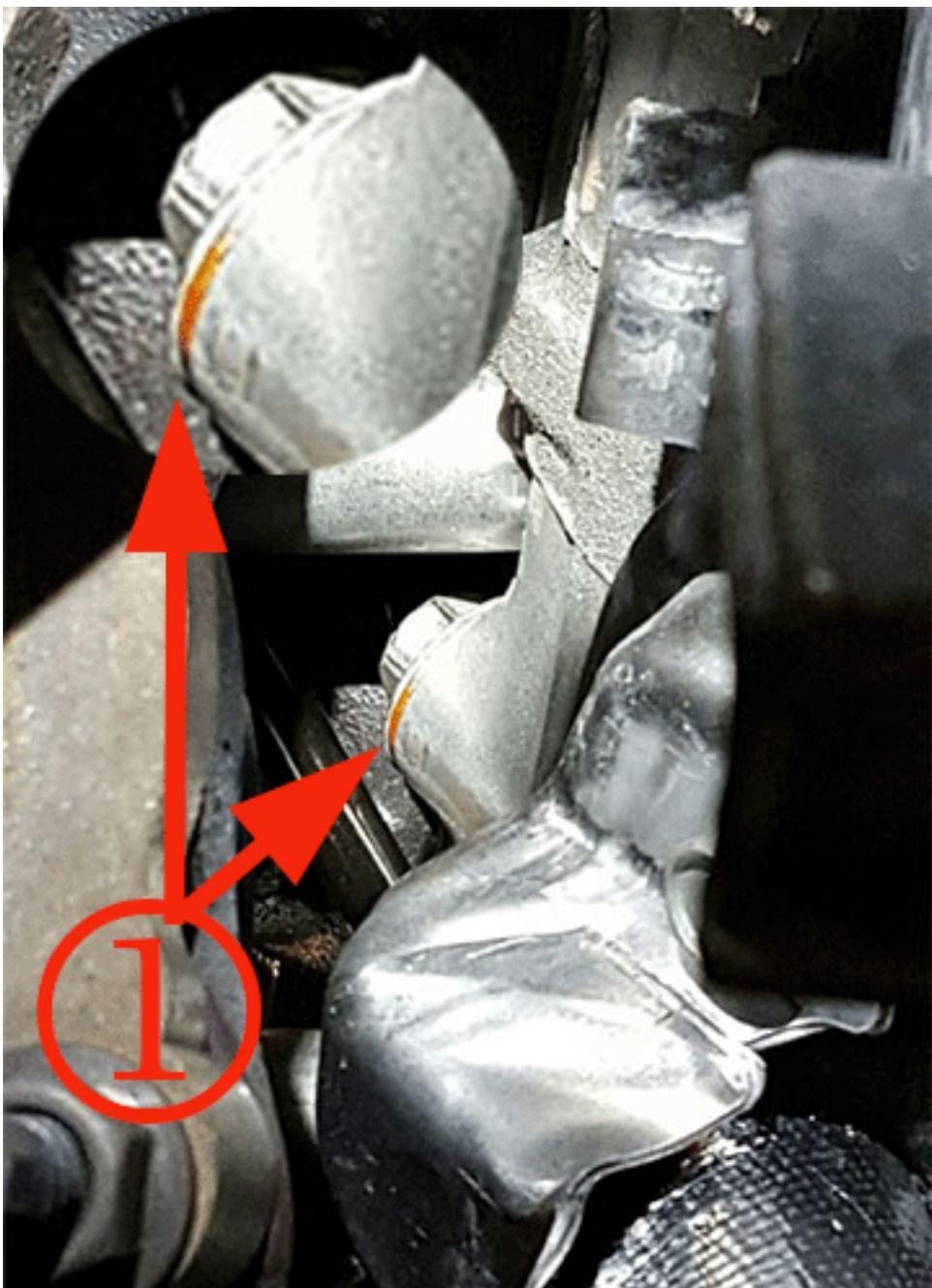
If a leak is found the head with the concern will need to be replaced.
