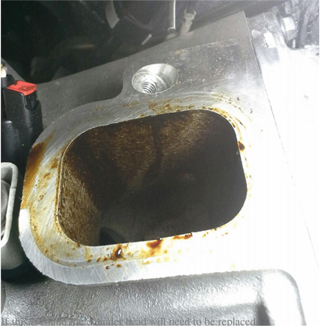
If this is found the cylinder head will need to be replaced
