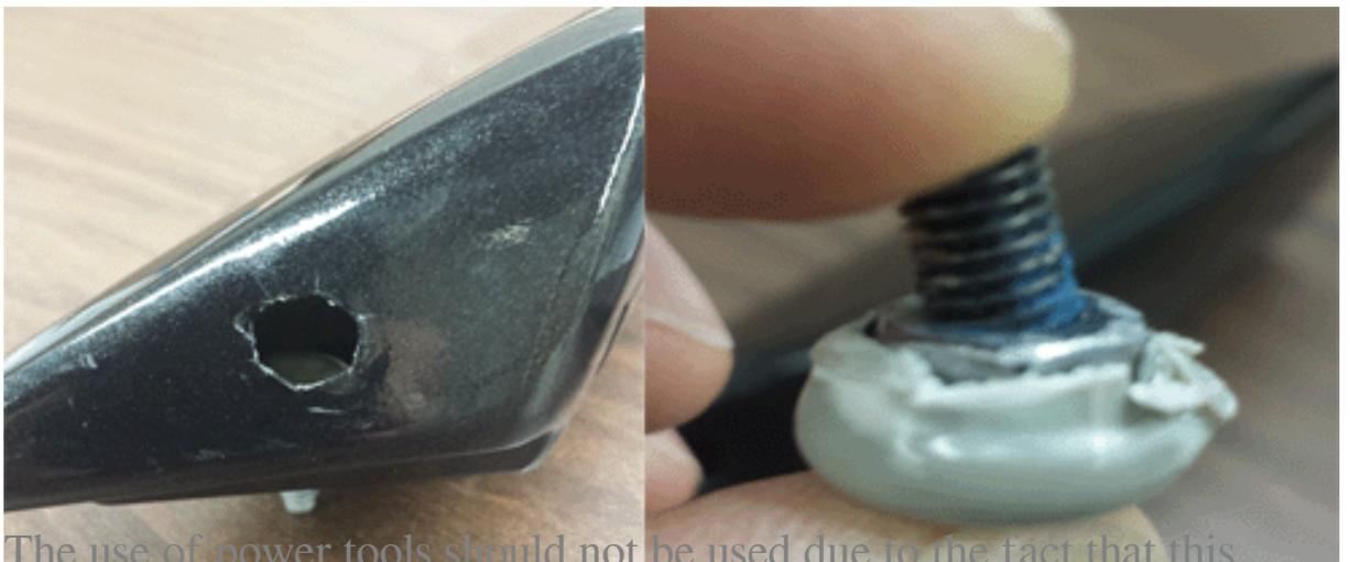
The use of power tools should not be used due to the fact that this could lead to damage to the fasteners and/or the spoiler.
