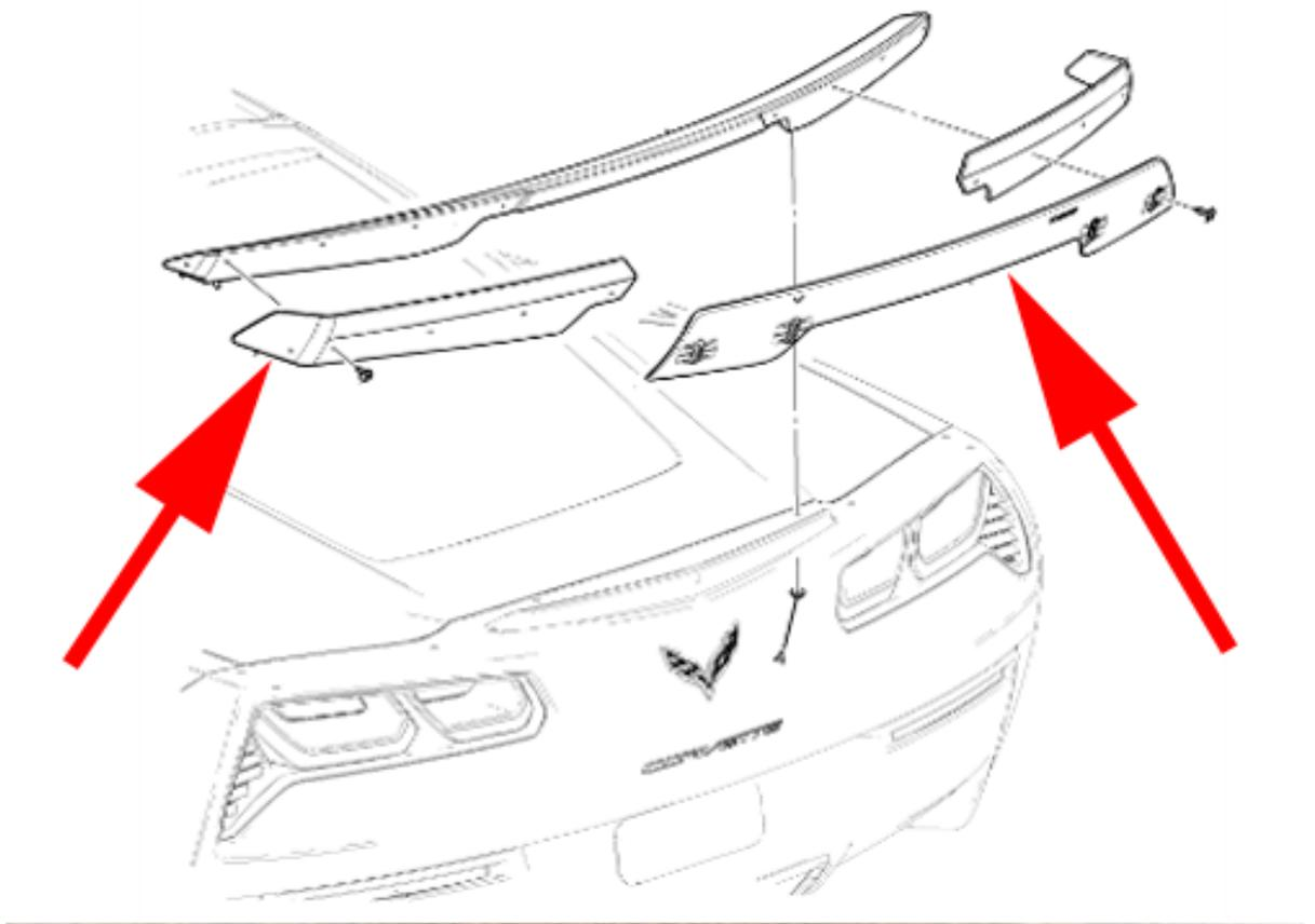
During the installation of the rear wicker bills that are fastened on the rear spoiler, some technicians may revert to the use of power tools to tighten the fasteners.
