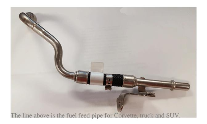
This line connects the chassis fuel line to the high pressure fuel pump.
