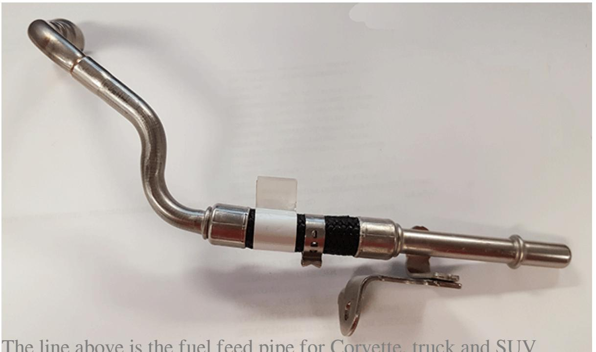
The line above is the fuel feed pipe for Corvette, truck and SUV.
