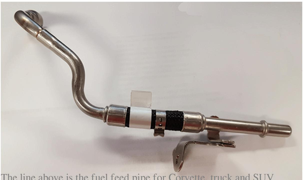
The line above is the fuel feed pipe for Corvette, truck and SUV.
