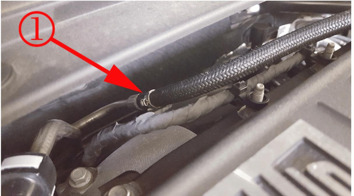
These pictures above shows the chassis fuel feed pipe for the LT4 supercharged ZL1 Camaro.
