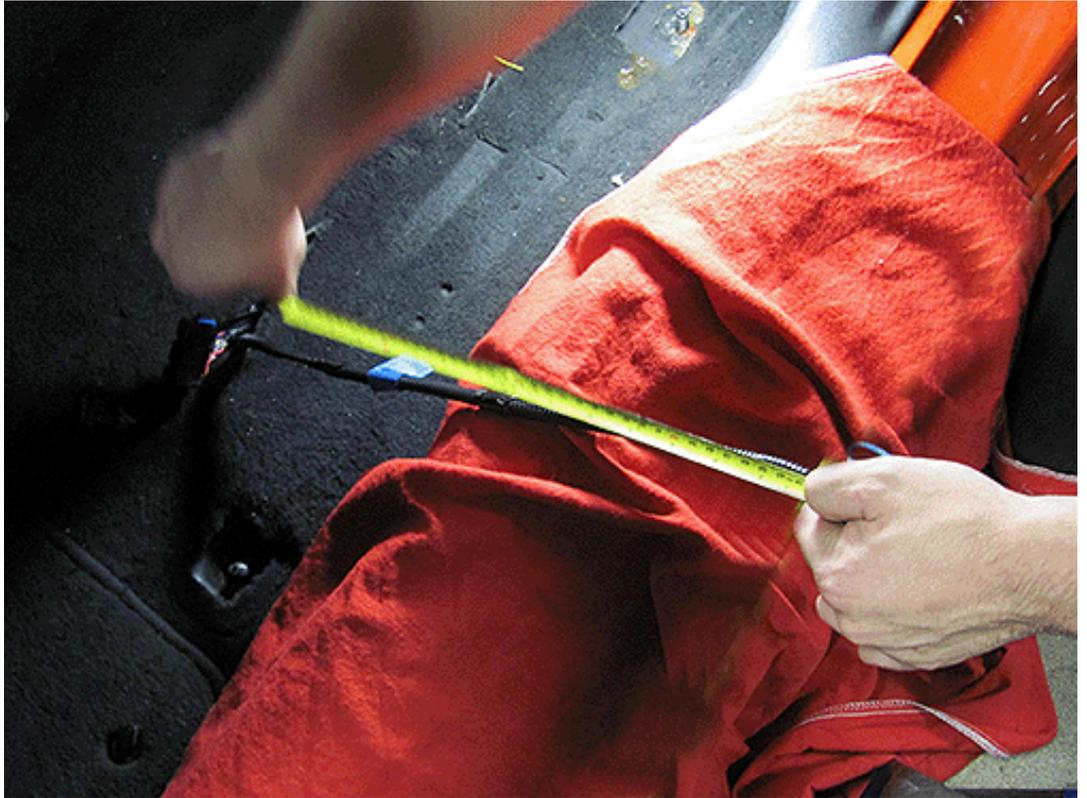
5. Measure 300mm (11.8 in) from the connector as shown.
