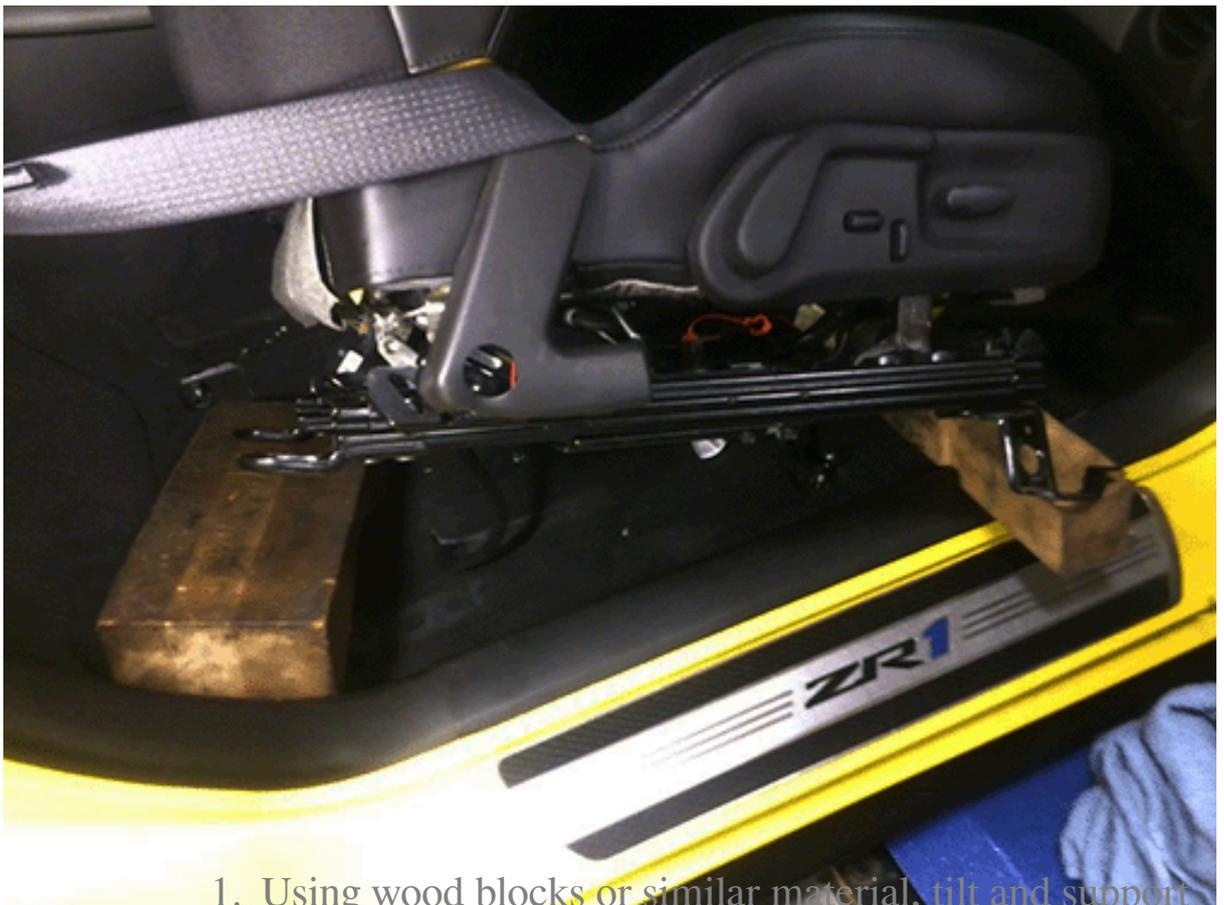
1. Using wood blocks or similar material, tilt and support the seat in the vehicle as shown.
