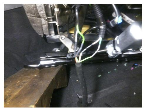
2. Center the heat shrink tube over all four splices and shrink/seal the heat shrink tube securely over the splice crimp and insulated wires.
