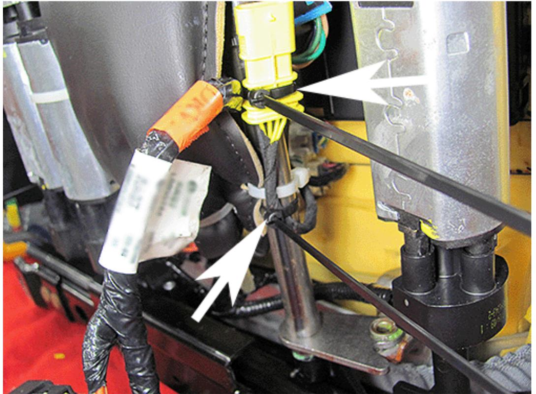
3. Secure the wire connector and harness to the FRONT seat cross bar using two cable ties.
