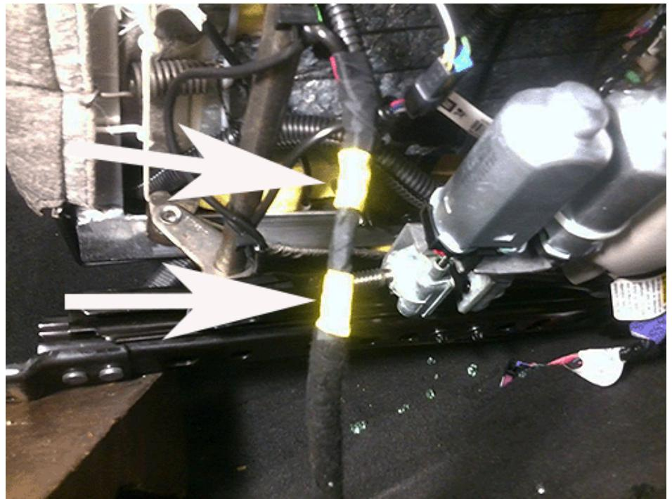
4. Wrap a section yellow electrical tape over the polyester electrical tape.
