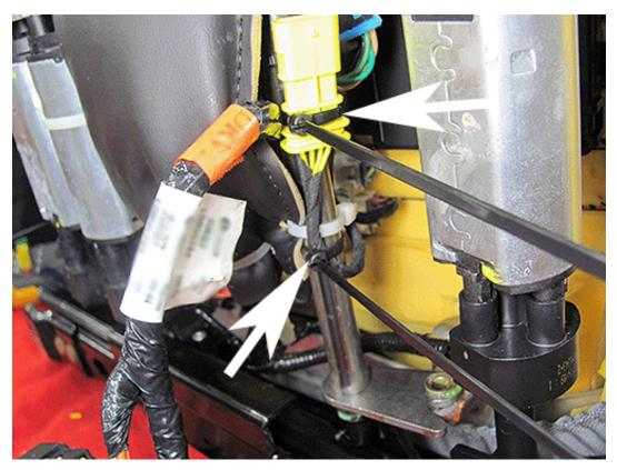
3. Secure the wire connector and harness to the FRONT seat cross bar using two cable ties.
