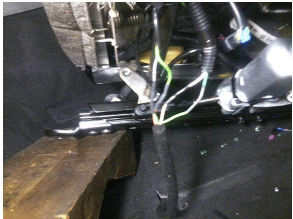
2. Center the heat shrink tube over all four splices and shrink/seal the heat shrink tube securely over the splice crimp and insulated wires.
