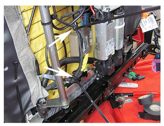
2. Secure the harness to the rear of the seat as shown.
