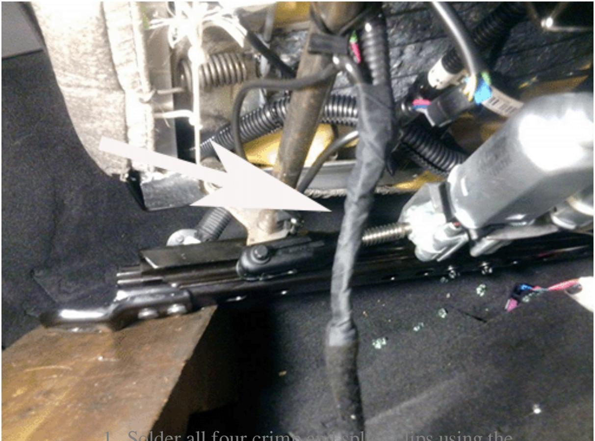
1. Solder all four crimp and split clips using the Ultratorch, part number J-38125-5, or another butane fueled soldering iron.
