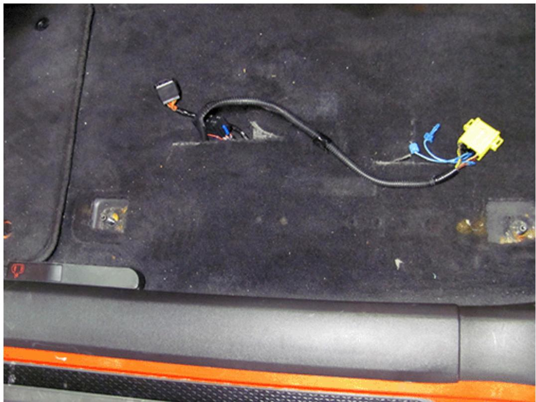
4. On the vehicle harness, pull the harness from under the carpet, to the front location as shown.
