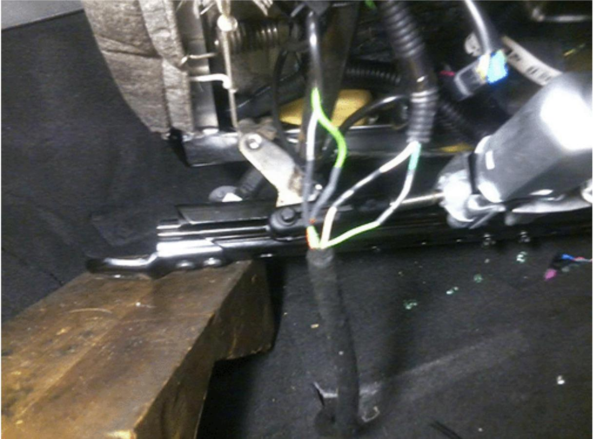
1. Crimp a splice clip over the joined wires using Special Tool J-38125-8, nest F. Verify the crimp quality. Repeat this crimp process on all four wire connections (2).
