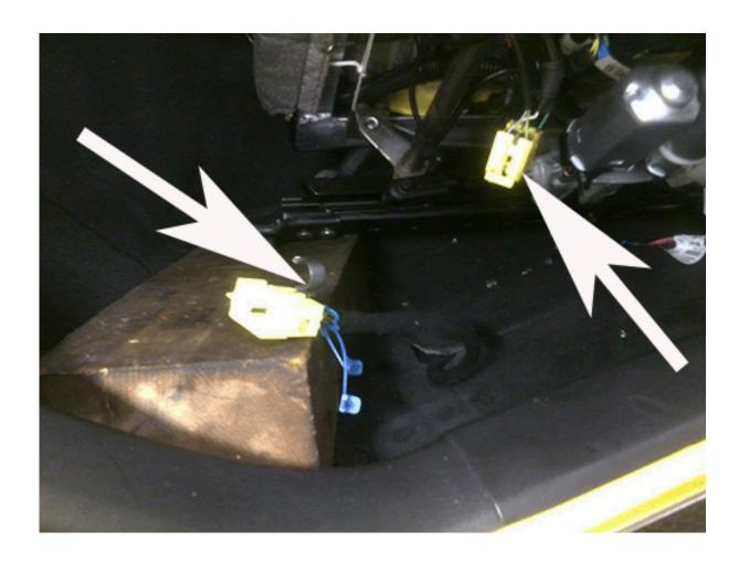
1. Locate the yellow harness connector. Disconnect the seat side connector from the vehicle side connector.
