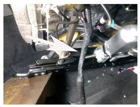
3. Wrap woven polyester electrical tape (PET) or equivalent anti-abrasion tape around the spliced section of seat harness.
