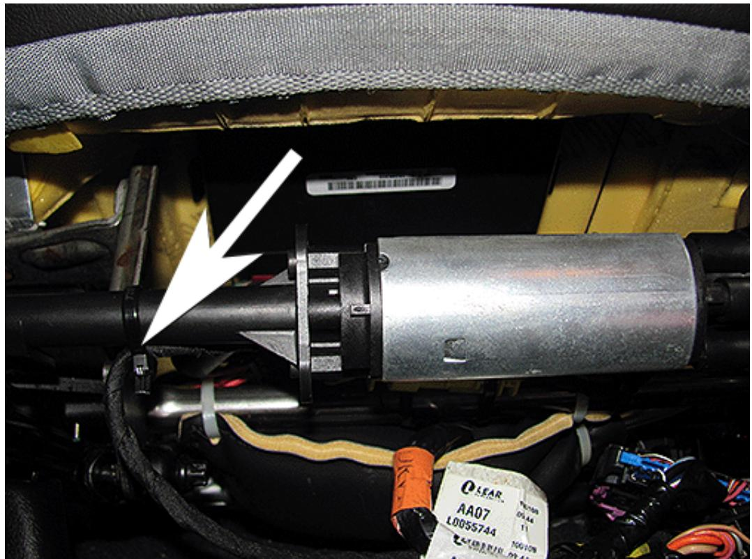
18. Using a cable tie, secure the harness to the FRONT seat cross bar.
