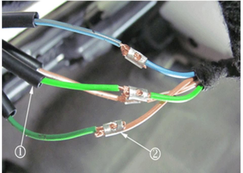
5. Add one approximate 38 mm (1.5 in) section of heat shrink tube to each of the four wires (1).
