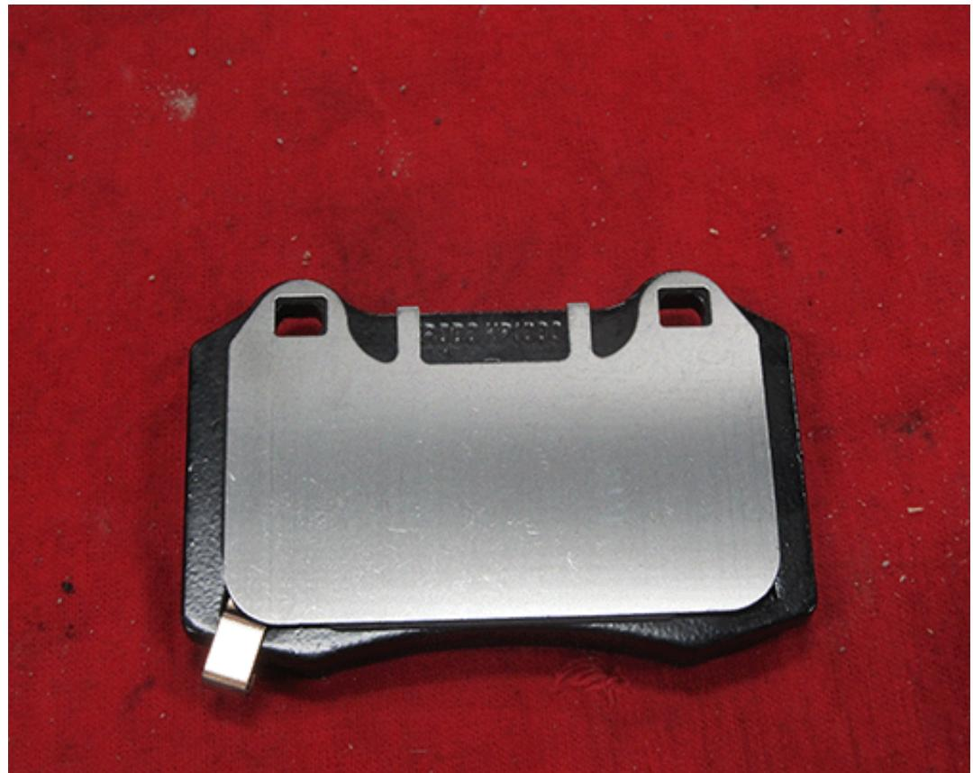
5. (Chevrolet SS Models Only) Apply a rectangular shape of copper paste in the center of the spacer before installing on the back of the pad.
