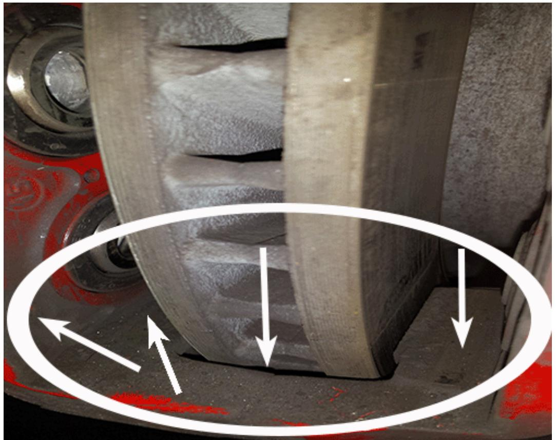
3. Using acrysol Kent Industries Part# P2005 or equivalent, wipe clean both ends of the abutment area on the front and rear pads and calipers.
