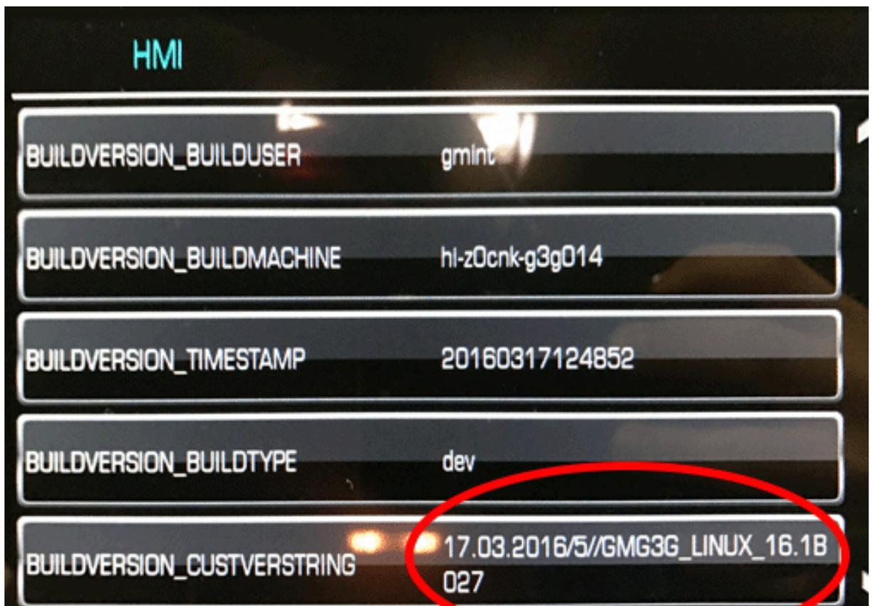
If the software is one of the following, reprogram the Human Machine Interface Control Module. Refer to *Human Machine Interface Control Module Programming and Setup* in SI.
