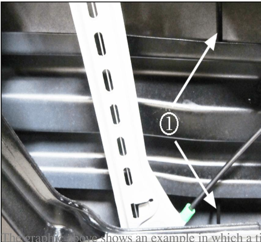
The graphic above shows an example in which a tie strap (1) was passed through a 15-20 cm (6-8 in) length gap where the adhesive was missing towards the center of the door.
