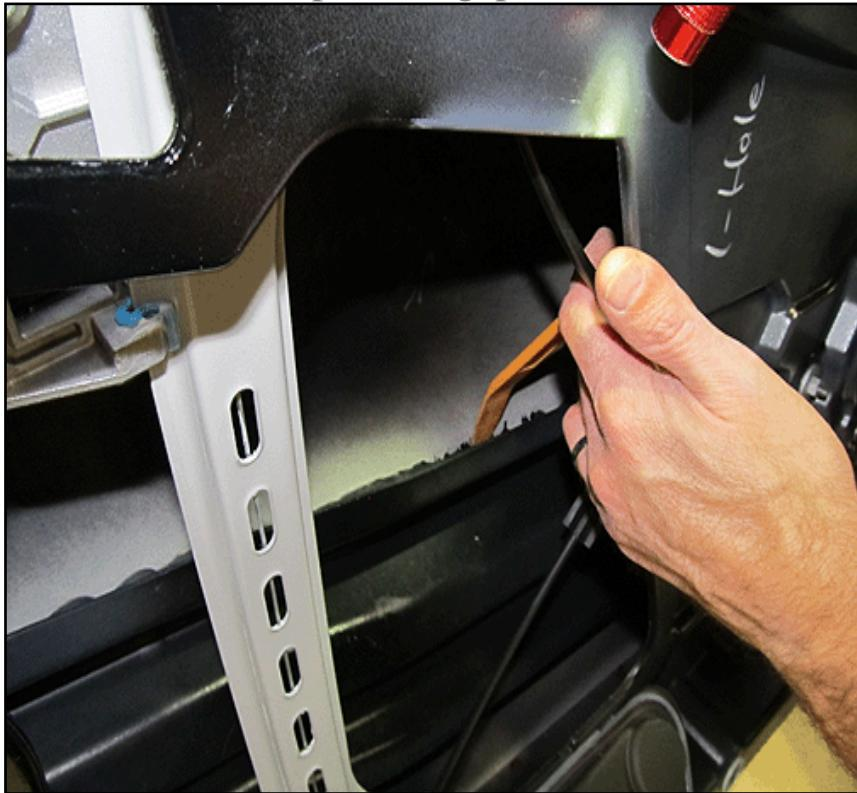
**Tip:** Use of a trim stick, or equivalent tool, may help to work the sealer into the gap.
