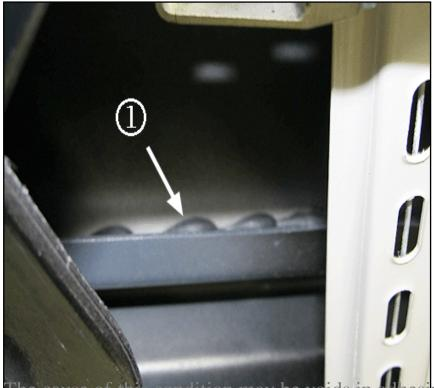
The cause of this condition may be voids in adhesive (1), leaving gaps between the inner door beam and the door skin.
