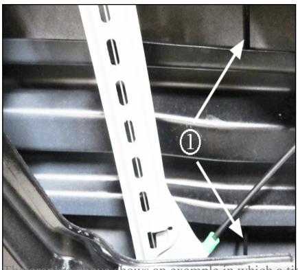
passed through a 15-20 cm (6-8 in) length gap where the adhesive was missing towards the center of the door.
