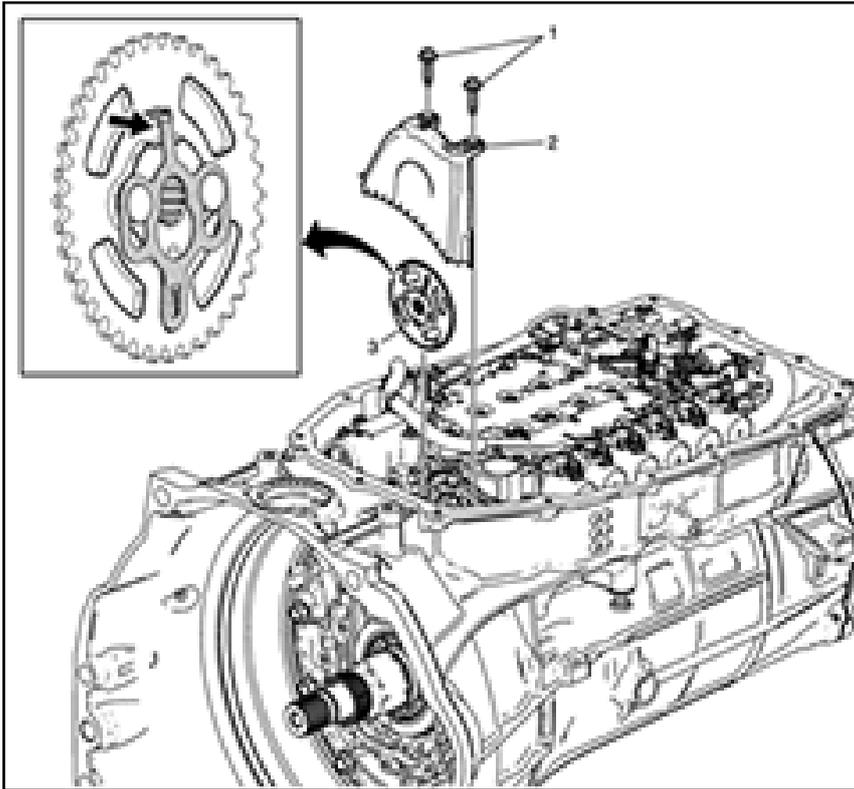
1. Using the DT-48285 Torx Plus socket, remove the two fluid baffle bolts (1) and fluid baffle (2). Discard the bolts.
