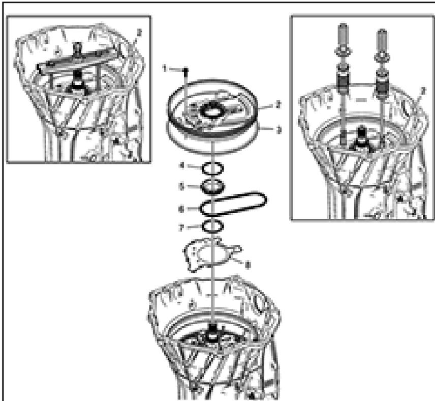
1. Remove the 11 front cover bolts (1). Discard the bolts. The bolts have a dry sealant on them and may only be used once.
