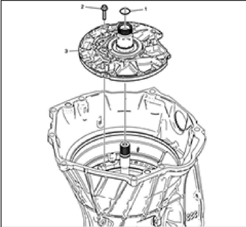
1. Remove the turbine shaft O-ring seal (1). Discard the seal.
