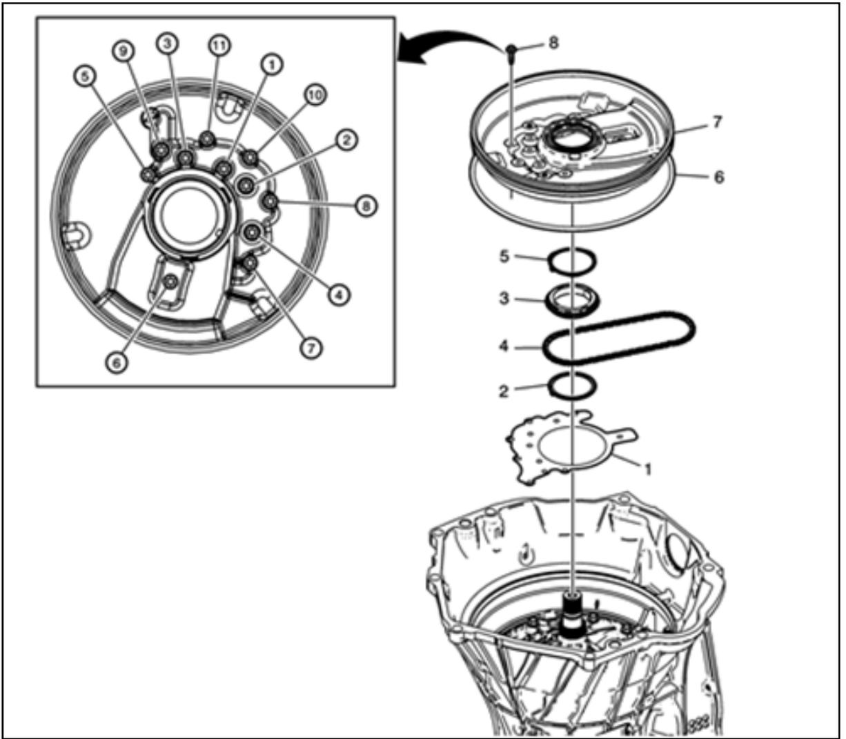
1. Install a NEW front support cover gasket (1).
