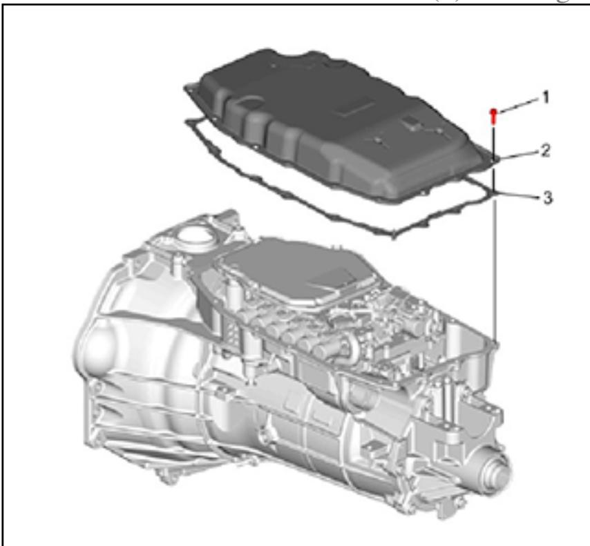
**Note:** The fluid pan gasket is reusable. Inspect the gasket to determine if it may be reused. If the gasket is stuck to the case or pan, it should be replaced.
