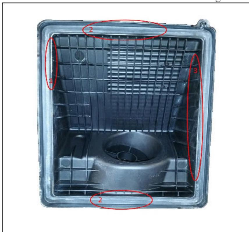
1. Inspect the air filter sealing surface for signs of not contacting the air filter seal (1, 2).
