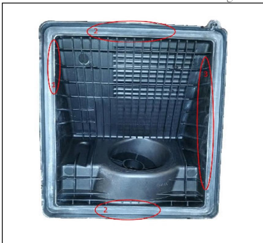
1. Inspect the air filter sealing surface for signs of not contacting the air filter seal (1, 2).
