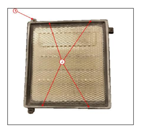
1. Inspect the all the air housing cover for any missing tabs and/or fasteners (1).
