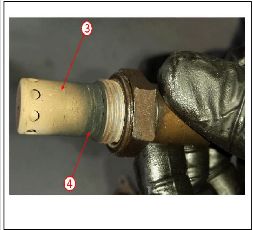
This may be caused by excessive sand and/or debris entering the air filter box and bypassing the seal of the air filter, due to not properly sealing, causing damage to the HO2 sensor element (3) and the catalytic converter to become blocked with sand and debris particles (1, 2).
