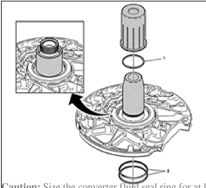
**Caution:** Size the converter fluid seal ring for at least 5 minutes after installation to obtain proper seal ring size. Failure to do so may cause internal transmission leaks and transmission damage.
