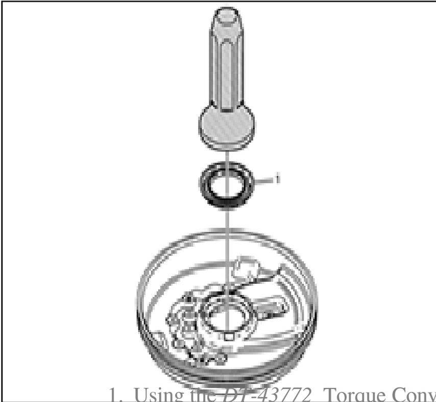
1. Using the *DT-43772* Torque Converter Seal Installer, install a NEW torque converter fluid seal (1) on the front cover.
