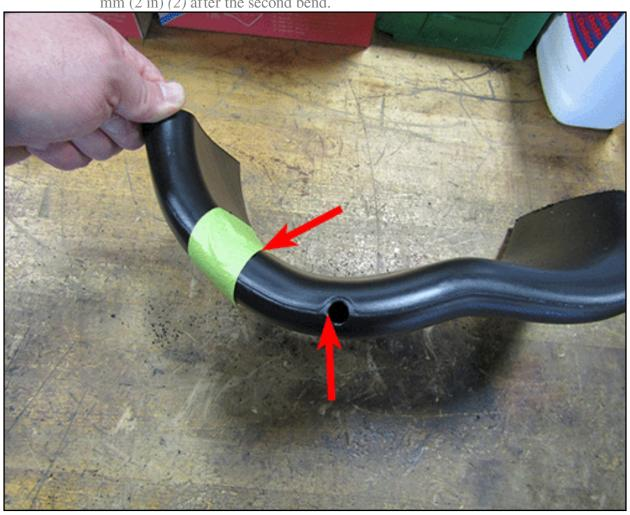
1. Measure 50.8 mm (2 in) up from the top of the hole. Mark and cut using a hack
