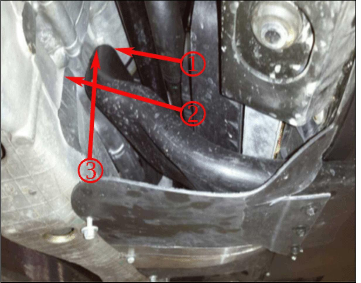
1. Once the part is riveted into place, dry fit to the car to make sure enough of the duct is cut to allow it to sit between the steering motor (1) and the lower rack (2).
