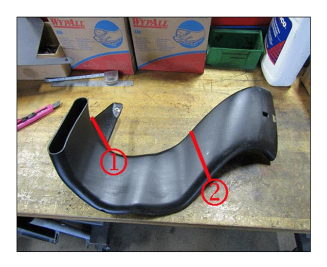
1. Using a hack saw, cut the support arm off (1) and the duct after measuring 50.8 mm (2 in) (2) after the second bend.
