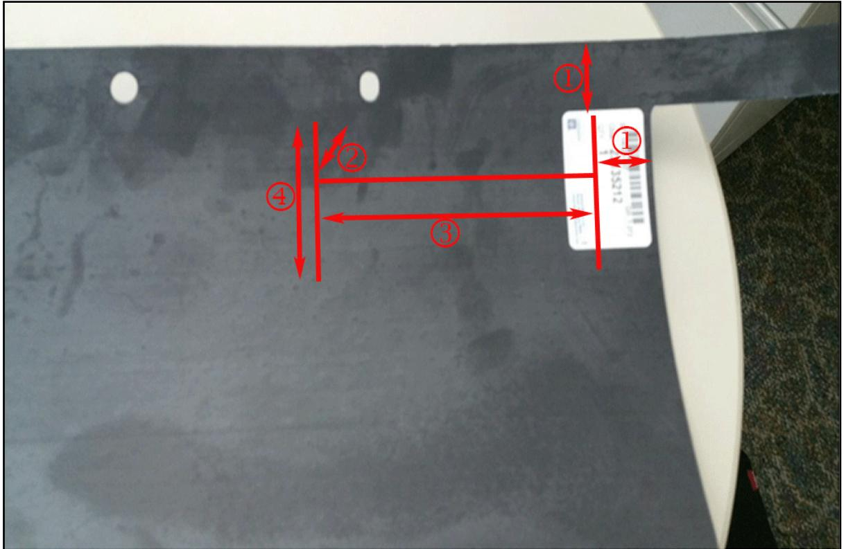
1. Place the new front compartment air deflector on a surface that can be used to cut on. Mark the dimensions of 25.4 mm (1 in) (1), 19.05 mm (.75 in) (2), 152.4 mm (6 in) (3), 50.8 mm (2 in) (4) as shown in the illustration above and cut using a box cutter.
