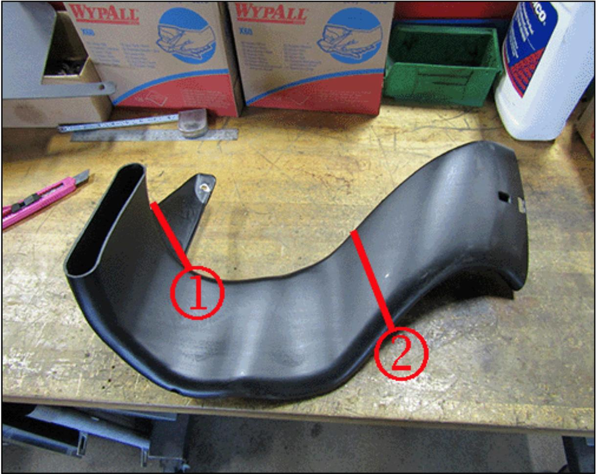
1. Using a hack saw, cut the support arm off (1) and the duct after measuring 50.8 mm (2 in) (2) after the second bend.
