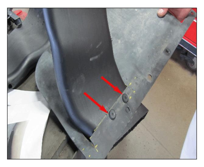
1. Place the cut duct into the slot. Make sure it comes out of the slot 25.4 mm (1 in). Using a 17/64" drill bit, drill 2 holes through the deflector and duct and rivet together.
