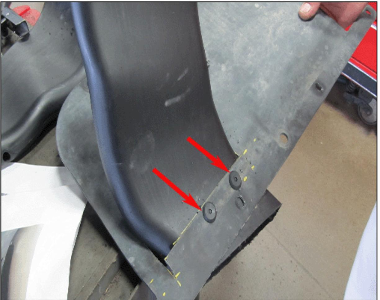
1. Place the cut duct into the slot. Make sure it comes out of the slot 25.4 mm (1 in). Using a  $17/64$ " drill bit, drill 2 holes through the deflector and duct and rivet together.
