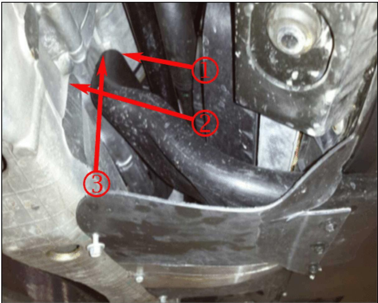
1. Once the part is riveted into place, dry fit to the car to make sure enough of the duct is cut to allow it to sit between the steering motor (1) and the lower rack (2).
