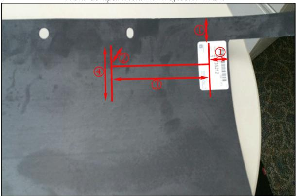
1. Place the new front compartment air deflector on a surface that can be used to cut on. Mark the dimensions of 25.4 mm (1 in) (1), 19.05 mm (.75 in) (2), 152.4 mm (6 in) (3), 50.8 mm (2 in) (4) as shown in the illustration above and cut using a box cutter.
