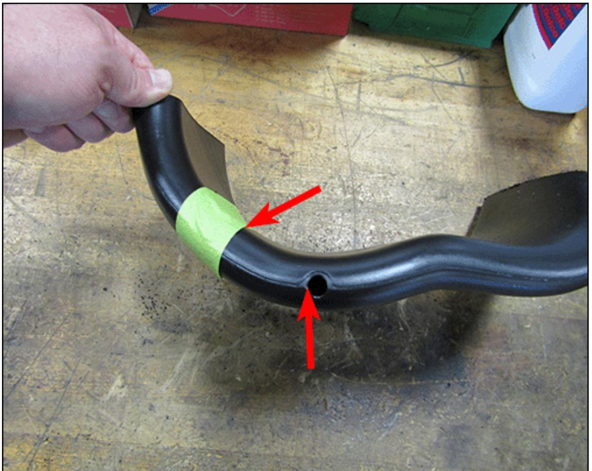
1. Measure 50.8 mm (2 in) up from the top of the hole. Mark and cut using a hack saw.
