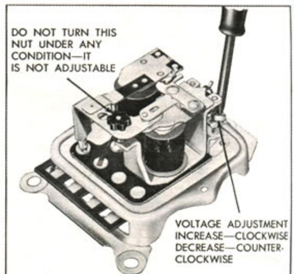
Fig. 1—Adjusting Regulator Voltage Setting
