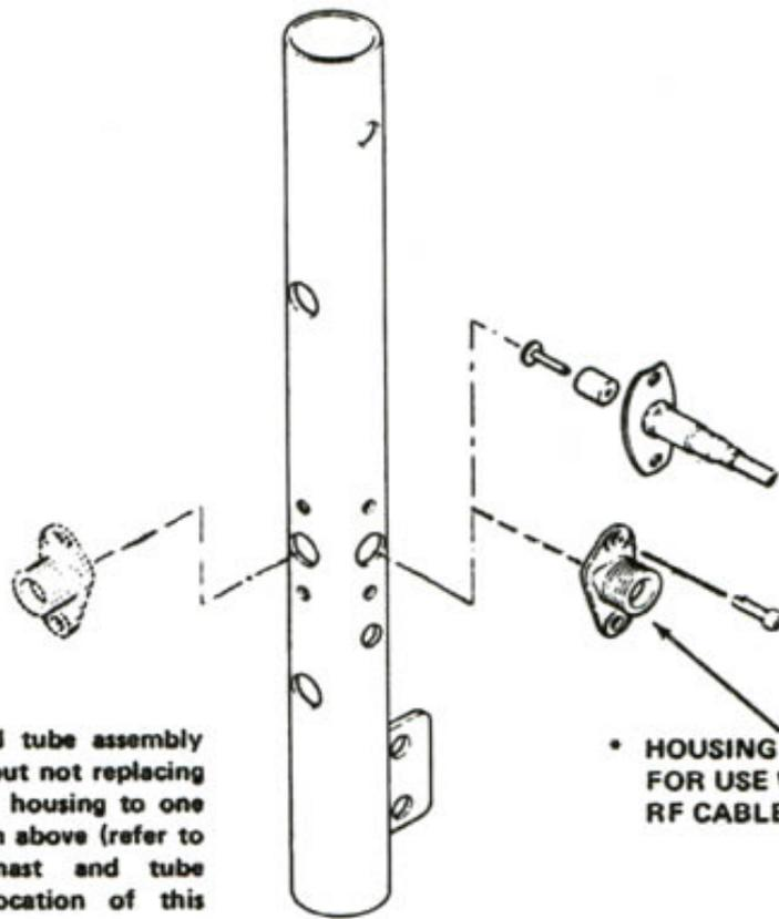
\*When replacing mast and tube assembly of your current antenna but not replacing the RF cable, attach this housing to one of the sets of holes shown above (refer to instruction sheet in mast and tube assembly package for location of this housing).
