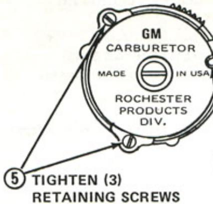
① **START THREE SELF-TAPPING SCREWS (NOTE: TIGHTEN SCREWS AFTER COVER INSTALLATION).**
