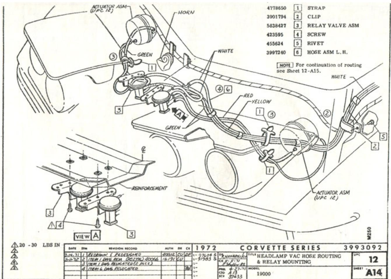
The schematic below shows the position of the headlight vacuum hose along the driver's side inner fender well:
