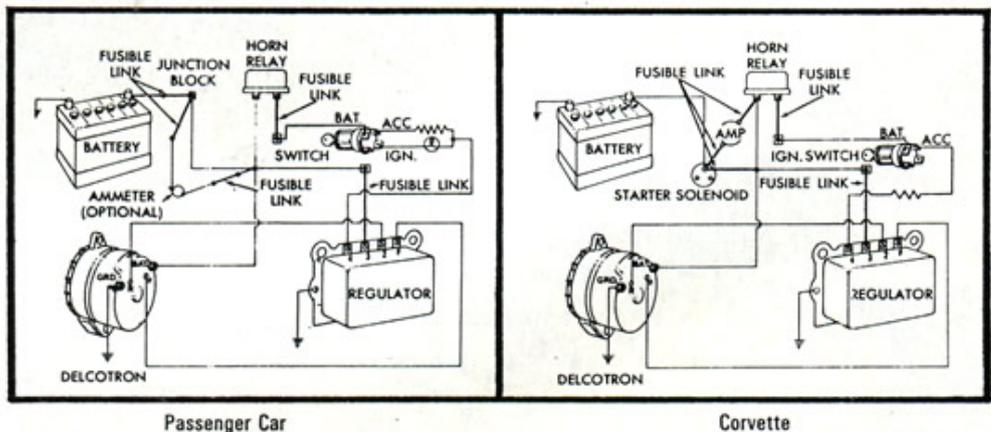
Fig. 1—Passenger Car Fusible Links
