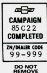
Each "Campaign Identification Label" is to be located on the radiator core support in an area which will be visible when the vehicle is brought in for periodic servicing by the owner.
