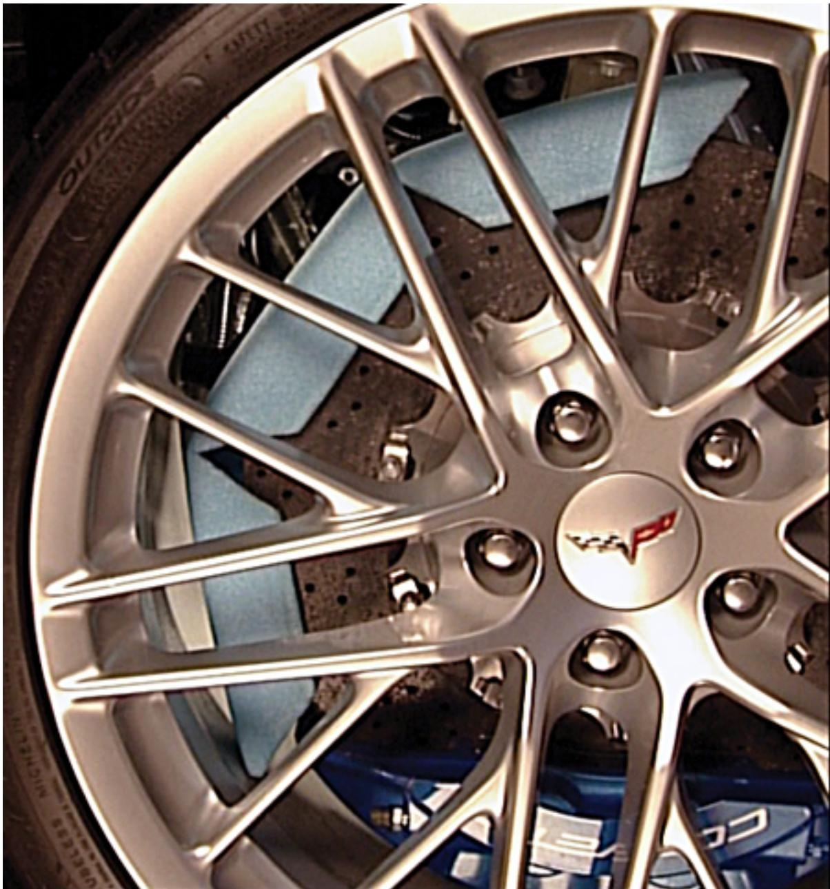
To prevent damage to the ceramic rotor, install a foam rotor protector before removing any wheel. Protectors can be installed through the spokes of the wheel.
