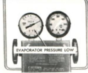
FIGURE 7—TXV STUCK CLOSED
