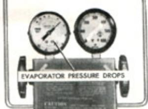
FIGURE 5—POA VALVE STUCK OPEN
