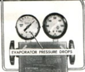
FIGURE 5—POA VALVE STUCK OPEN
