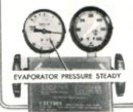
FIGURE 6—POA VALVE STUCK CLOSED
