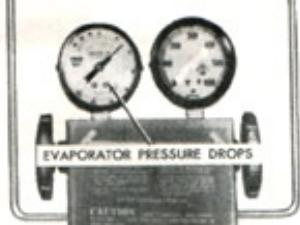
FIGURE 5—POA VALVE STUCK OPEN
