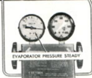
FIGURE 6—POA VALVE STUCK CLOSED
