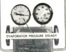
FIGURE 6—POA VALVE STUCK CLOSED
