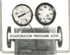
FIGURE 7—TXV STUCK CLOSED
