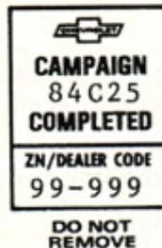
Each "Campaign Identification Label" is to be located on the radiator core support in an area which will be visible when the vehicle is brought in for periodic servicing by the owner.
