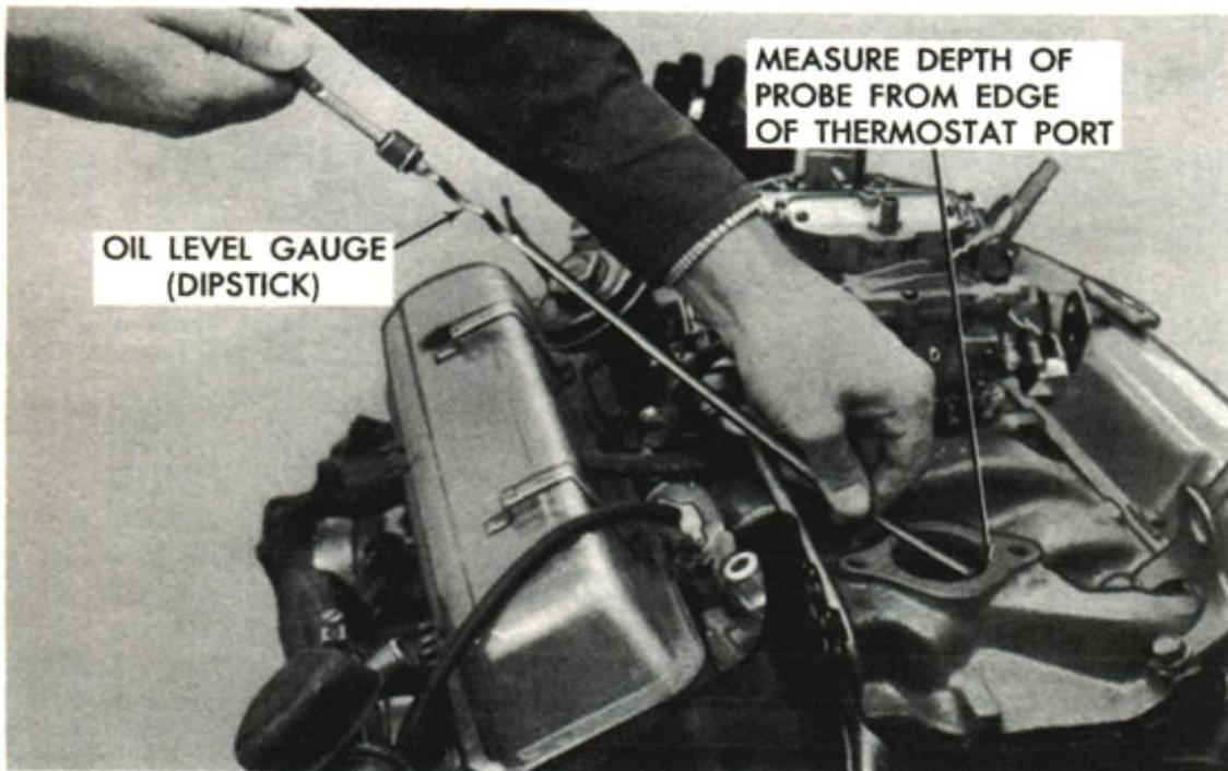
**INSPECTION PROBE OF COOLANT EXIT PORT**
