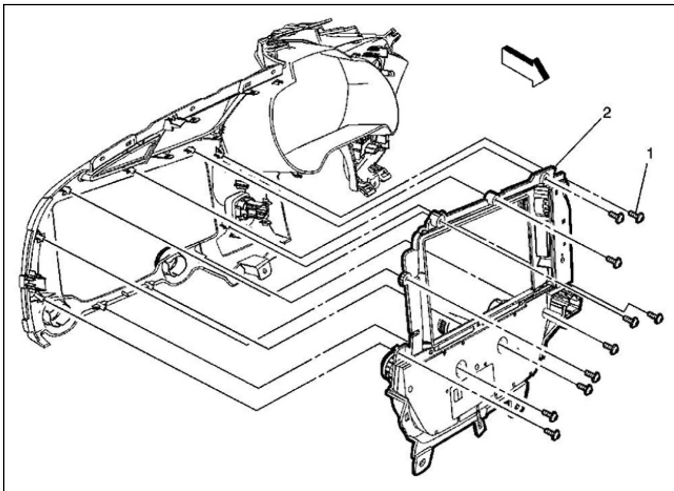
To remove the assembly, the instrument panel trim plate must first be removed. Pull the radio knobs straight off to allow the radio control to be separated from the trim plate. Refer to the appropriate Service Information for the complete repair procedure.
