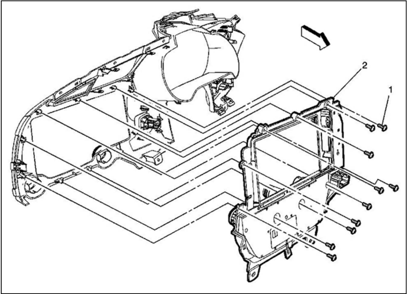
To remove the assembly, the instrument panel trim plate must first be removed. Pull the radio knobs straight off to allow the radio control to be separated from the trim plate. Refer to the appropriate Service Information for the complete repair procedure.
