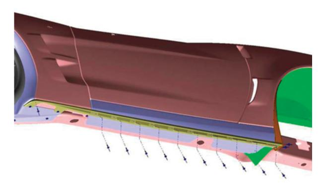
**TIP:** Due to the length of the rocker moldings, have an assistant help hold the moldings in place to avoid breakage.
