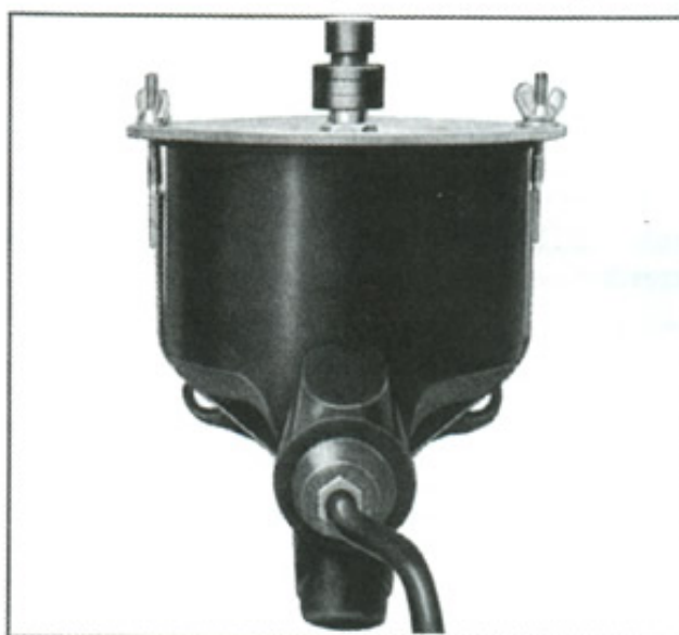
Fig. 30—J-21994 Pressure Bleeder on Master Cylinder
