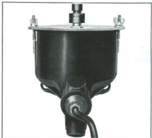
Fig. 30—J-21994 Pressure Bleeder on Master Cylinder
