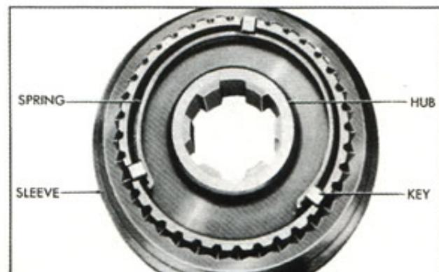
Fig. 10—Clutch Assembly
