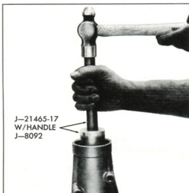
Fig. 11—Removing and Installing Rear Extension Bushing
