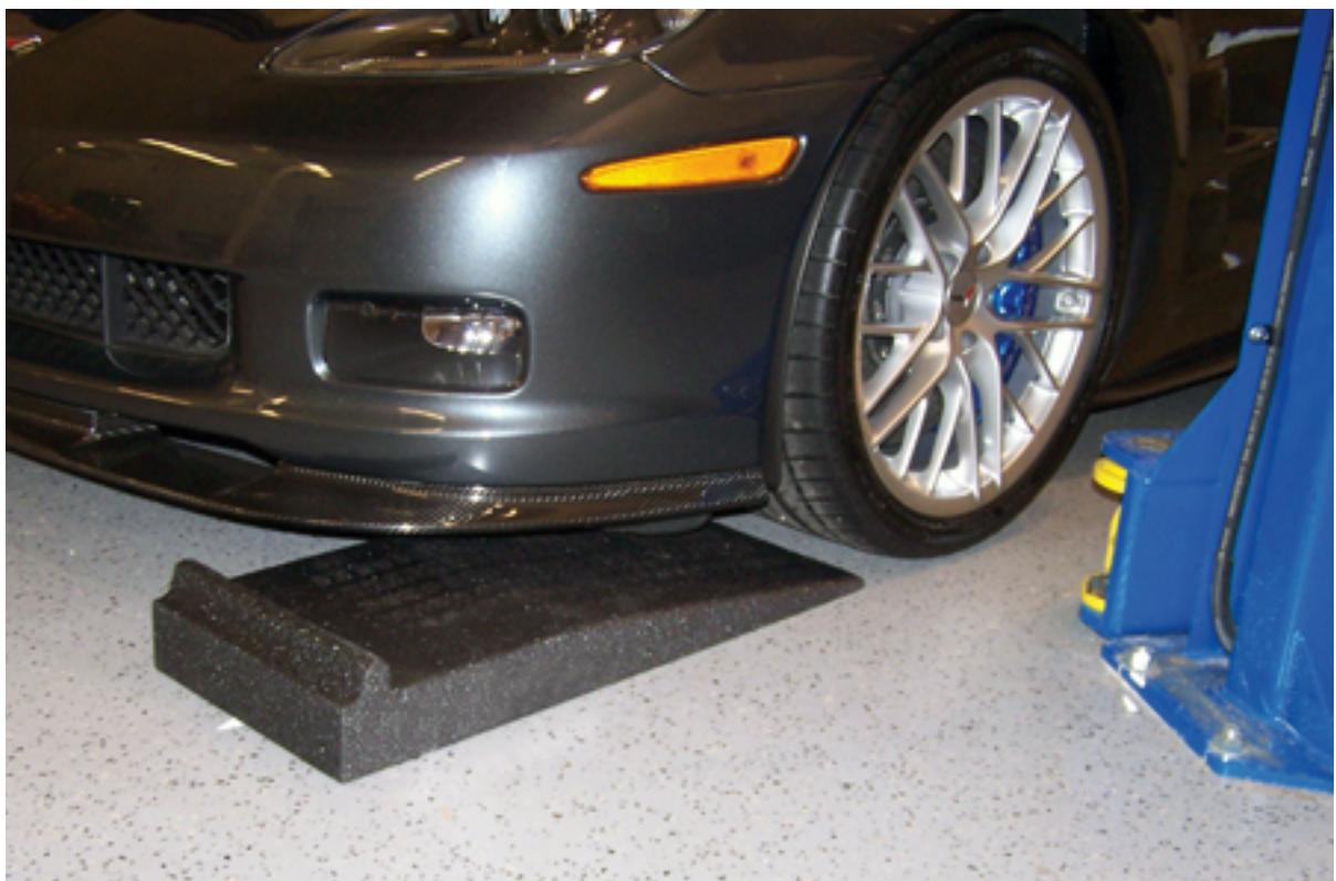
On a lift with telescoping lift arms, check the height of the outer (larger) portion -- it may contact the rocker panel even if the smaller (inner) portion clears (fig. 22) .
