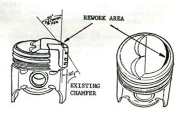
Reworking Piston Dome - 1961 Corvette Models Equipped With Fuel Injection
