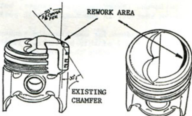
Reworking Piston Dome - 1961 Corvette Models Equipped
