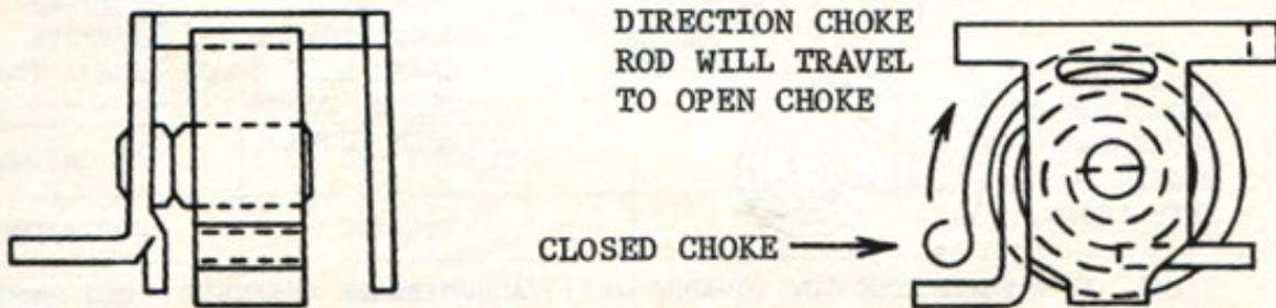
FIG. II - CHOKE THERMOSTAT ASSEMBLY - 327 V-8 (275 HP)
