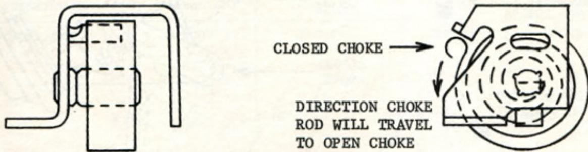
FIG. I - CHOKE THERMOSTAT ASSEMBLY - 283 V-8
