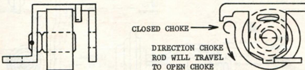
FIG. III - CHOKE THERMOSTAT ASSEMBLY - V-8 exc. 283 & 327 (275 HP)
