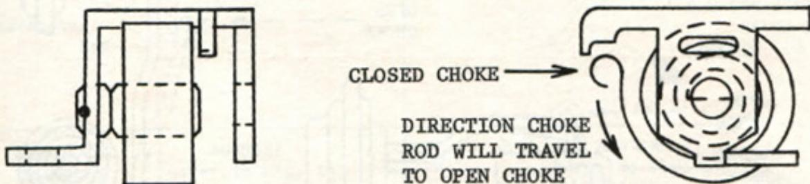
FIG. III - CHOKE THERMOSTAT ASSEMBLY - V-8 exc. 283 & 327 (275 HP)
