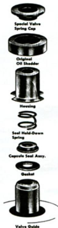
The new **SKINNER OIL SAVERS** are capsule-type valve stem oil seals specially designed to end excessive oil consumption problems at lowest possible cost. Easily installed *without pulling the cylinder head*, they provide a tight, dependable closing, with a hold-down spring keeping the capsulated seal firmly in place.
