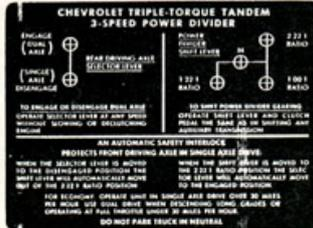
Triple Torque Power Divider
