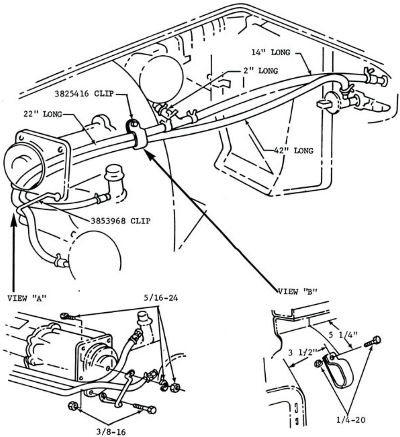
FIGURE II - HEATER HOSE ROUTING
