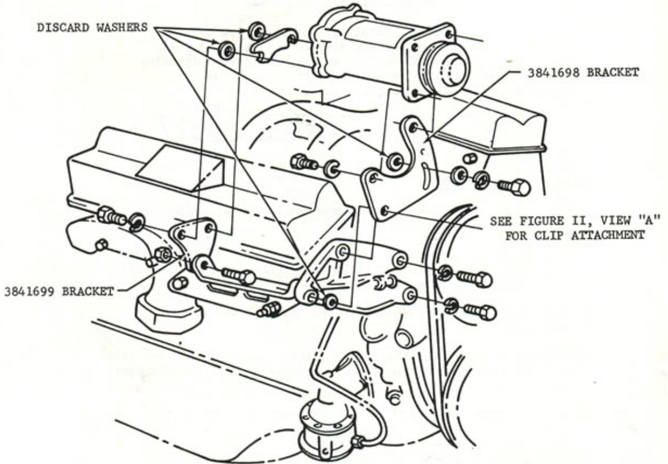
FIGURE I - A/C COMPRESSOR BRACKET MOUNTING
