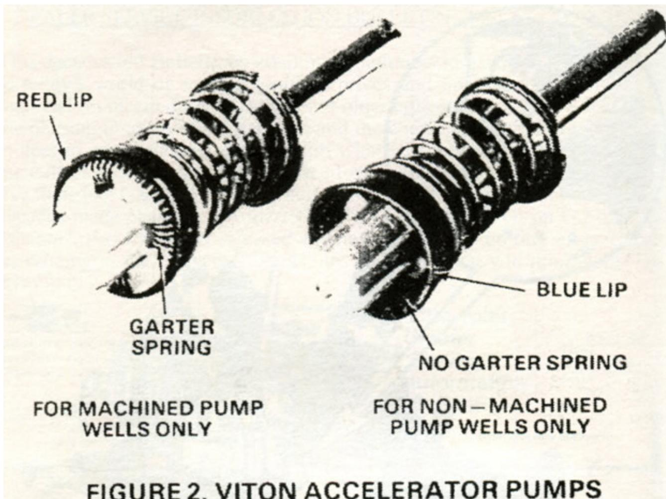
**FIGURE 2. VITON ACCELERATOR PUMPS**
