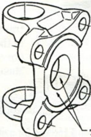
FIGURE 3 - DRIVESHAFT FLANGE
