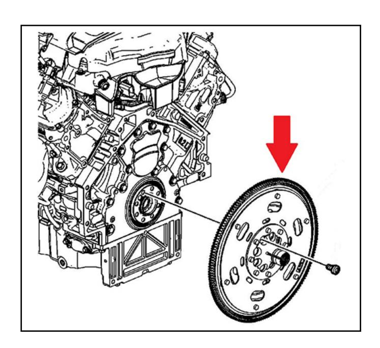
**TIP:** Check that the pinch clamp bolt is tight before replacing the front flex plate. The loose bolt condition results in the same noise. This is an easy check before starting a major service procedure.
