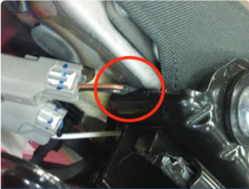
**Fuel fill valve Heater element harnesses near the rear inboard corner of the seat assembly**
