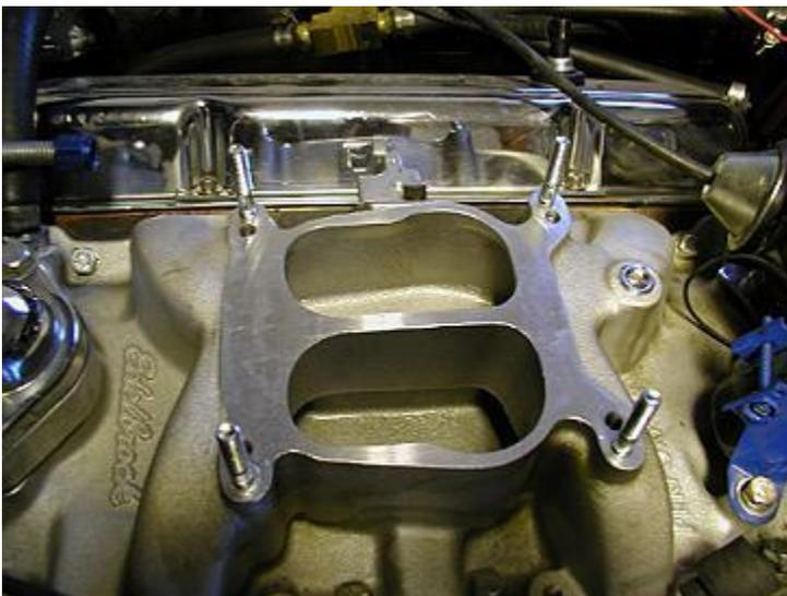
Using the 1/4" thick insulating gasket under the heat shield requires use of long mounting studs. Note also that the vacuum fitting in the manifold to the rear of the carb has been removed and a flush allen-head pipe plug has been installed to clear the BG rear float bowl and allow installation of the jogged shield.
