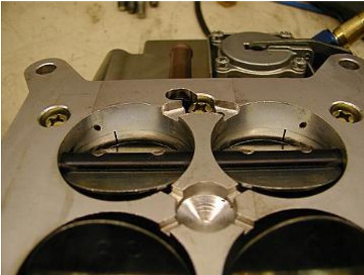
Throttle blades cracked open to show the vertical transition slots. These slots start metering fuel as you come off idle and as you go into the main discharge circuit. If too much of the slots are exposed, idle mixtures will be incorrect. .020" of the slots should be exposed below the edge of the throttle blades.
