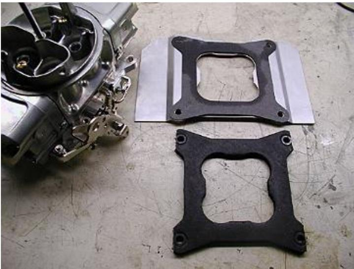
In order for the “jogged” shield to clear the base gasket, the gasket “ears” must be trimmed. Shown here is a trimmed base gasket that will allow the bent shield to fit properly.
