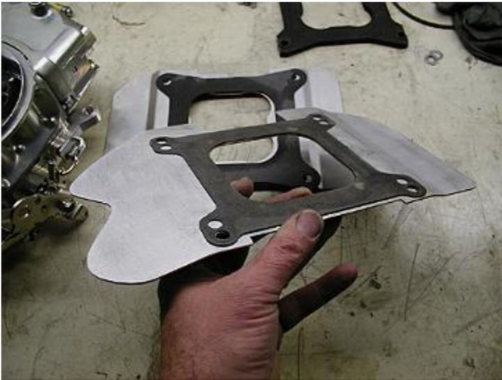
Shields can be made in many ways. Shown here is the custom shield that I use on my own car. It's fabricated from a piece of aluminum sheet stock. Note forward and rear edges bent down to clear accel pump levers.
